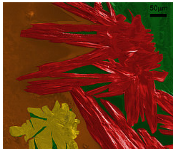
Figure 4.2. This scanning electron microscopy image is of the protein ubiquitin mixed with a MALDI matrix from which samples for atom probe tomography were prepared. The image will help researchers choose regions for further detailed atomic-scale characterization of these proteins by atom probe tomography analysis.
