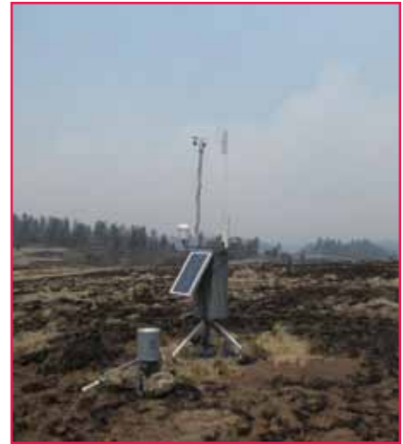
Deployed to a grassy area during the Wallow Fire, AZ, this IRAWS was subjected to a burnover but continued to operate properly. Photo: Alan Hester, BLM, June 2011.
