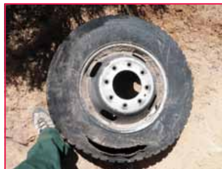
The initial attack squad vehicle's outside-rear dual tire that caught fire when parked in the black on the 2010 Plug Hat Fire. Photo: Plug Hat Fire, Damage to Government Vehicle Non-Serious Accident Investigation Report, 2010.
