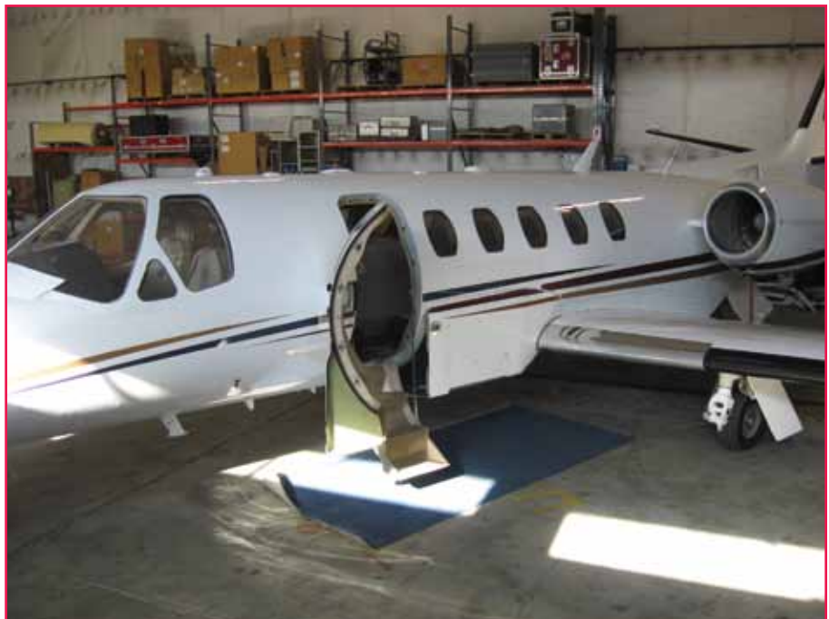
The NIROPS scanner is mounted in the bottom of the aircraft fuselage. In this Citation aircraft, it is located just to the right of the steps. Photo: Ken Frederick, National Interagency Fire Center.
