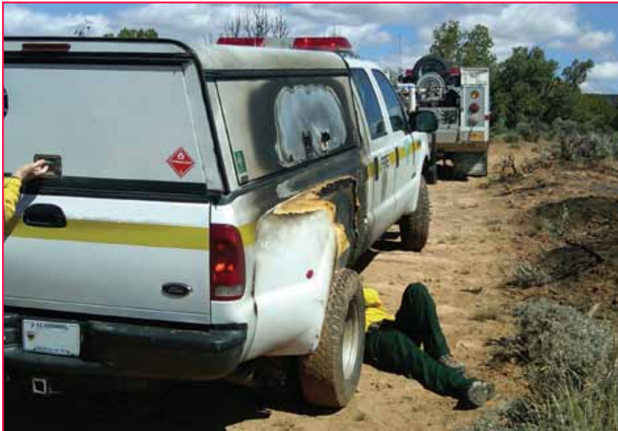
Both vehicles that caught fire while parked in the black during the 2010 fire season were carrying flammable liquids. Photo: Plug Hat Fire, Damage to Government Vehicle Non-Serious Accident Investigation Report, 2010.
