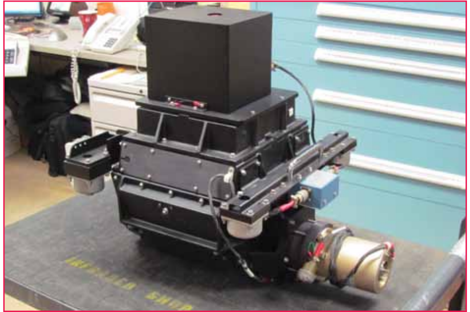
NIROPS uses a Kennedy line scanner to record infrared data from 10,000 feet (3,048 m) altitude. This compact piece of equipment performs a critical job for incident management teams. Photo: Ken Frederick, National Interagency Fire Center.
