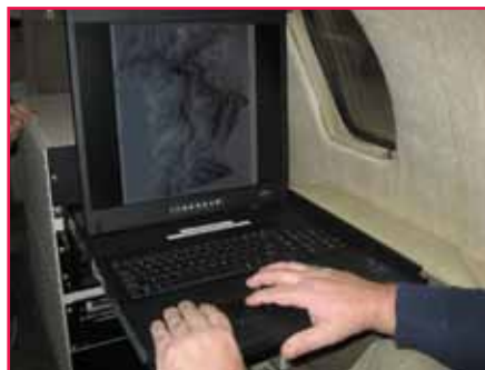
An infrared technician checks a scanner image on the data processing platform inside NIROPS’ Citation jet. Photo: Ken Frederick, National Interagency Fire Center.
