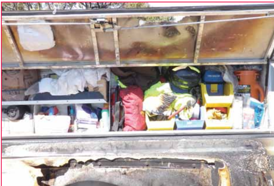
Fire damage spread in the initial attack squad vehicle compartment from the tire that ignited while the vehicle was parked inside the burn perimeter—in the black—on the 2010 Plug Hat Fire. Photo: Plug Hat Fire, Damage to Government Vehicle Non-Serious Accident Investigation Report, 2010.
