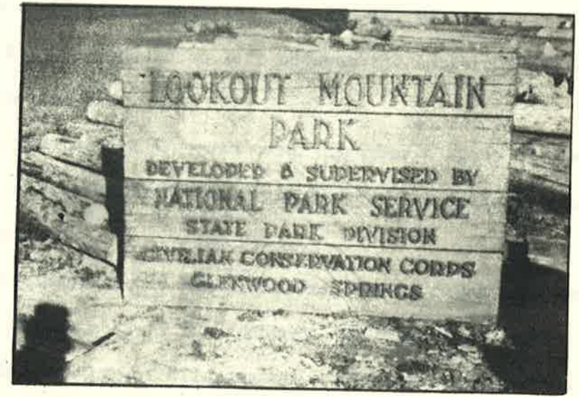
METAL LETTERS. Letters cut from steel plate with welding outfit and mounted on a wooden panel with cap screws. The heads of the cap screws are welded to the back of the letters.
