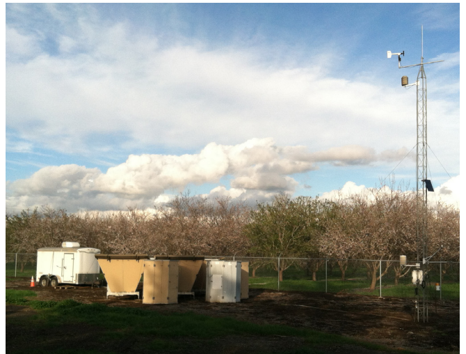
Instruments at an HMT field site in Chico, California including a wind profiler and meteorological tower. (Credit: Clark King, NOAA)
