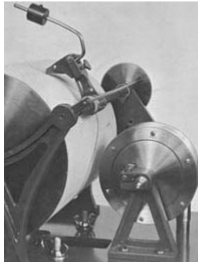
This is one of the earliest mechanical pen and ink strip recorders for measuring tidal levels. Click the image for a larger view.
