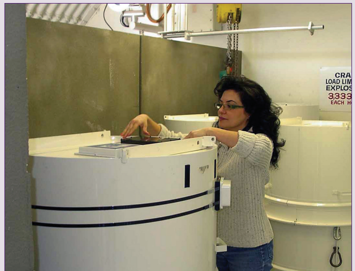
LLNL researcher attaching an RFID tag to a container used in a technology demonstration.
