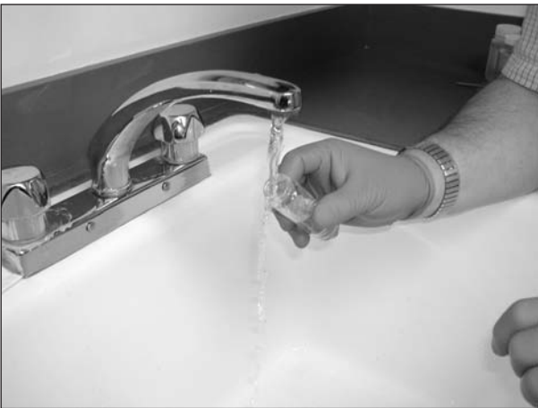
Tilting the vial to prevent formation of air bubbles.
