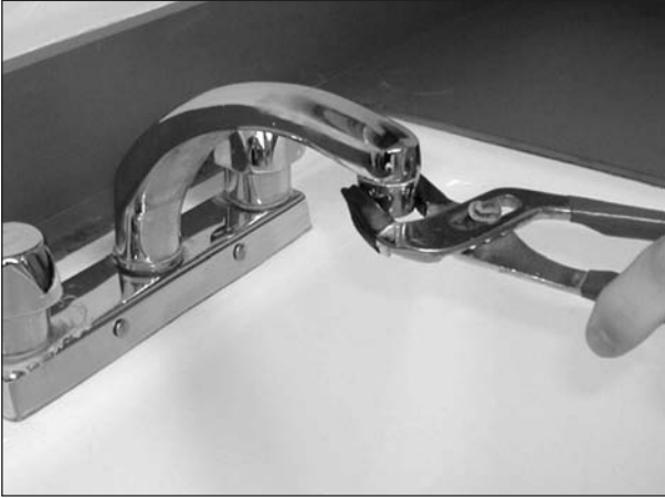
Removing aerator from faucet before starting to sample
