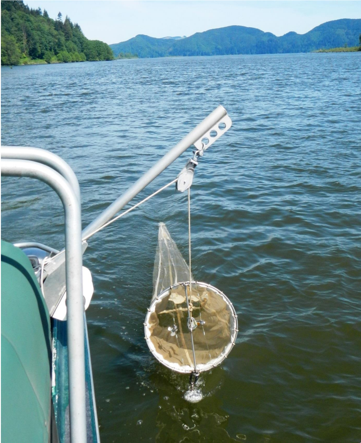
Figure 3. Photograph of the plankton net setup deployed to collect eulachon smelt eggs and larvae. Image shows the setup when two General Oceanic flow meters were mounted to the frame.
