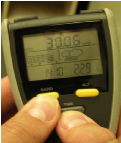
Figure 4. Press Baro and Time together for 2 seconds to start calibration
