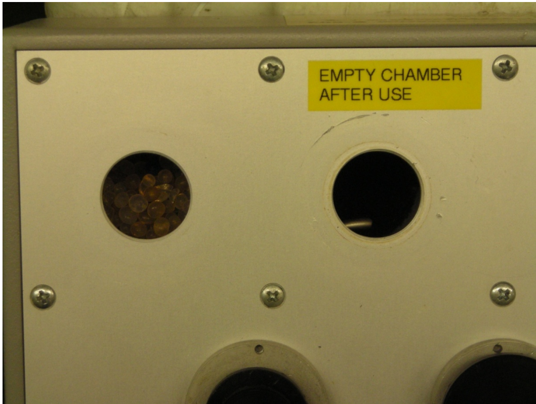
Figure 3. Inspect desiccant and water reservoirs for proper media levels
