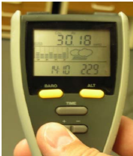
Figure 5. Press “+” or “-” to adjust the pressure reading up and down
