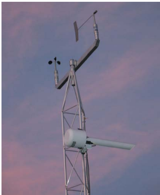
Figure 19. Climatronics Meteorological System. Climatronics Meteorological Tower Showing Wind Speed Sensor, Wind Direction Sensor, Cross-arm and 9-meter Aspirated Temperature Shield containing T1 Temperature Probe and RH Probe.
