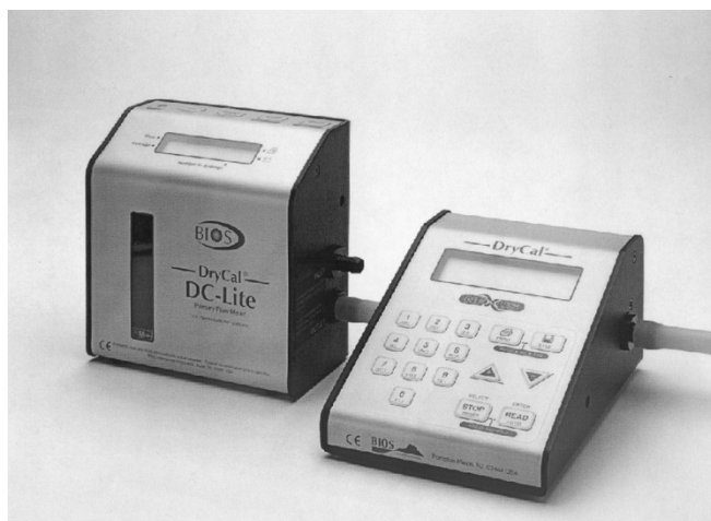
Figure 2. DC-Lite (left) and Nexus (right) flow calibration standard
