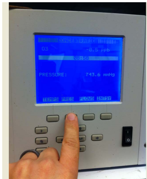
Figure 17. O 3 Analyzer Display of Cell Pressure
