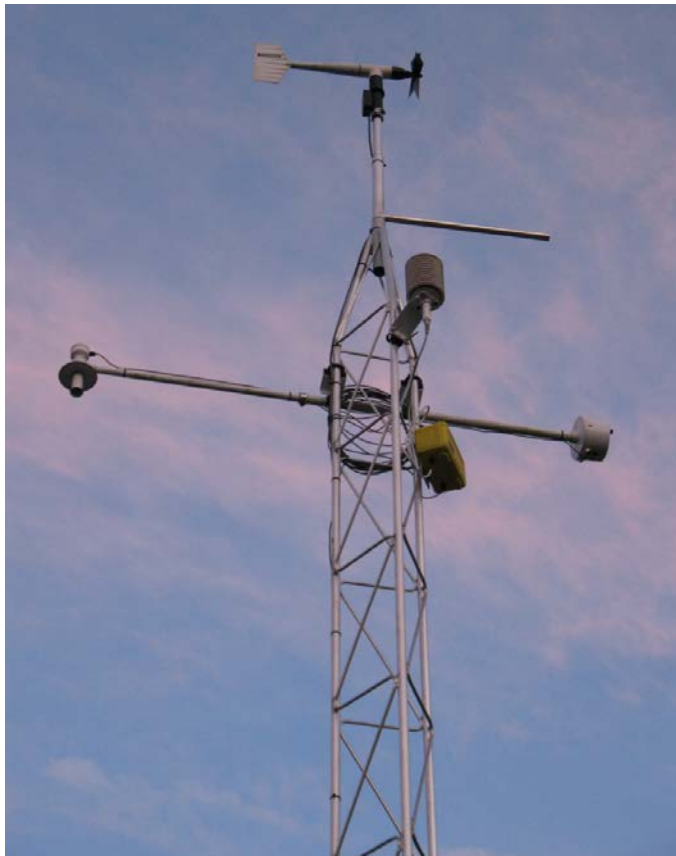
Figure 27. RM Young Meteorological System: (from top to bottom) Meteorological Tower with Wind AQ, Directional Cross-Arm, Gill Aspirated Shield for RH Probe, 9-m Aspirated Temperature Sensor Shield and Waterproof RH Circuit Card "Otter" box.
