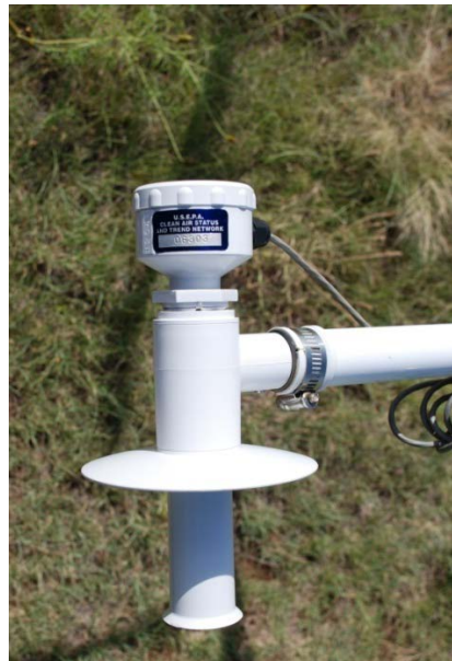
Figure 32. RM Young Temperature Probe Installed in Aspirated Shield.
