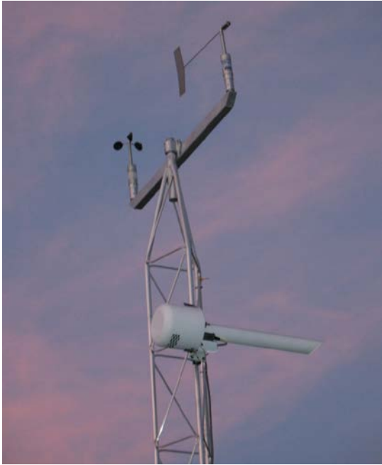
Figure 1. Climatronics Meteorological System. Climatronics Meteorological Tower Showing Wind Speed Sensor, Wind Direction Sensor, Cross-arm and 9-meter Aspirated Temperature Shield containing T1 Temperature Probe and RH Probe.
