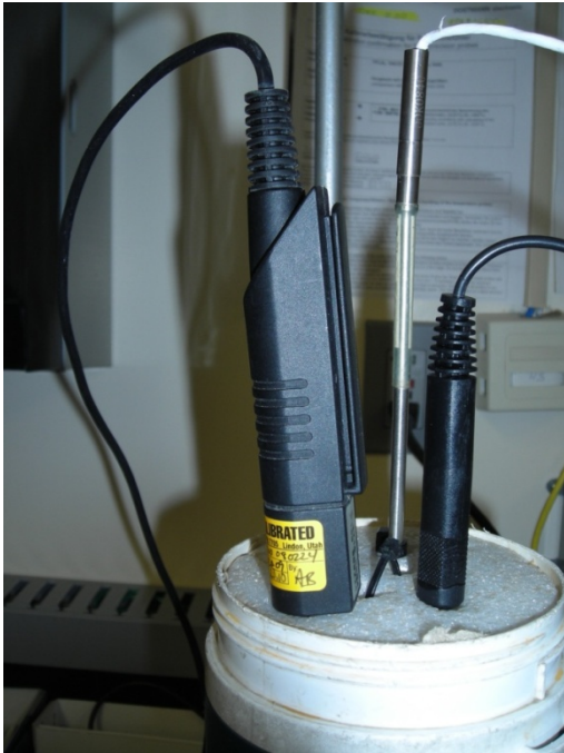
Figure 3. Dostmann probe (left), Eutechnics transfer probe (middle) and Extech probe (right) immersed in stirring bath. More than one temperature transfer device may be certified simultaneously.
