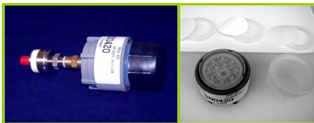
Figure 1-2 Three-Stage Filter Pack
