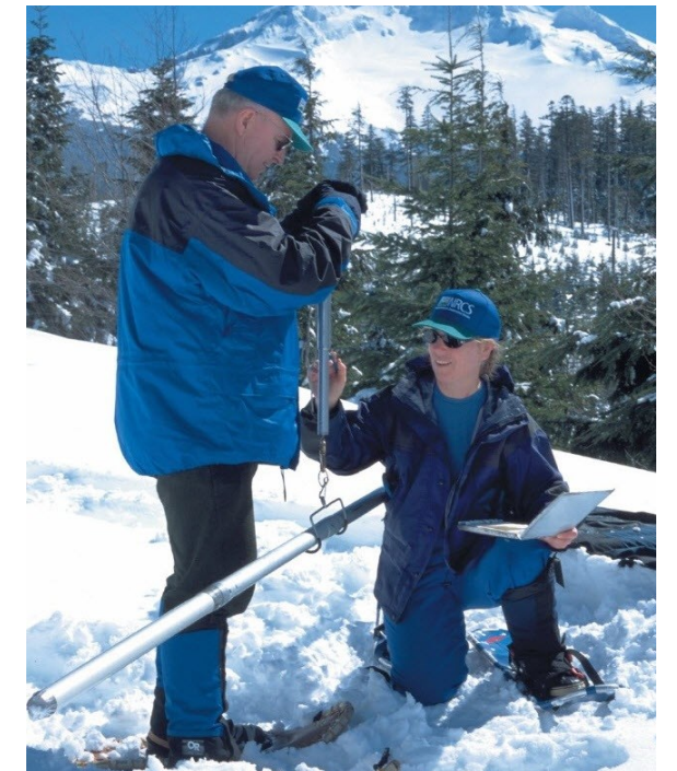
Using a snow scale to measure snow water equivalent of mountain snowpack.
