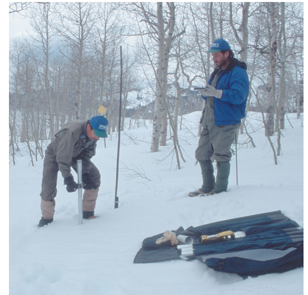
Extracting a core sample of the snowpack using a snow tube.
