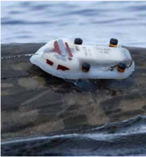
Close-up photograph of multi-sensor tag attached to a humpback whale via suction cups.
