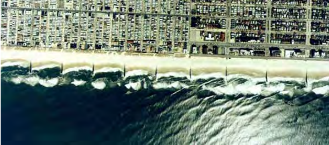
Figure 7.12. Groin field in Long Beach, New York (New York Sea Grant photo)
