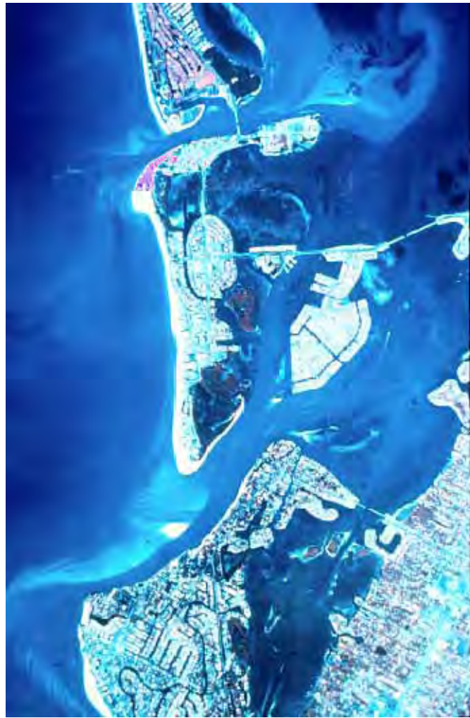
Figure 5.19. Two tidal inlets on the southwest Florida coast (New Pass and Big Sarasota Pass). Lido Key is the barrier island between the two inlets. Net longshore sand transport is to the south.
