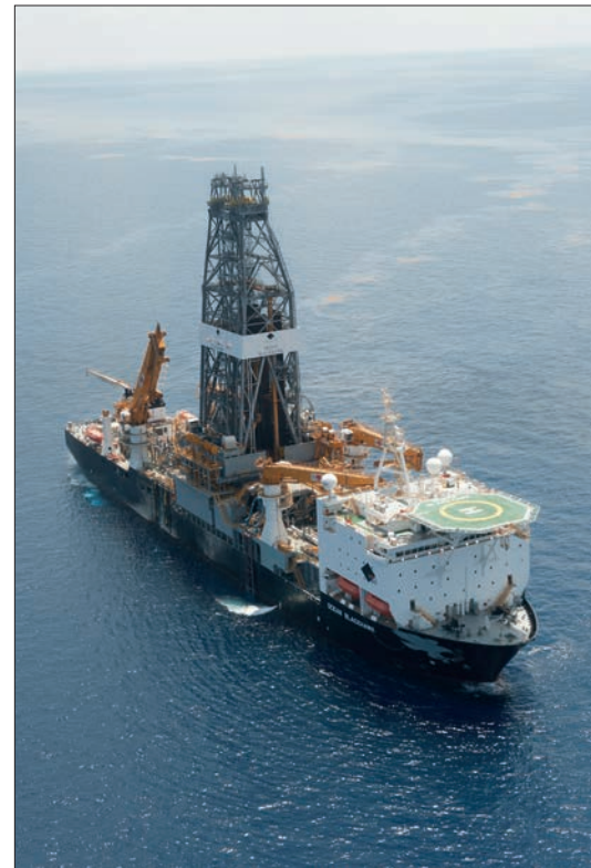
This dynamically-positioned drillship, the Ocean BlackHawk, is capable of operating in water depths up to 12,000 ft. and can drill to a depth of 40,000 ft. Owned and managed by Diamond Offshore Drilling, the Ocean BlackHawk is currently operating in the U.S. Gulf of Mexico.
