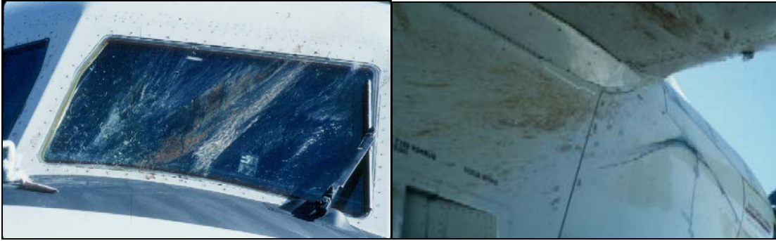
Figure 2. E-2 bird strike with western gulls destroyed the aircraft. Pilots escaped without injuries.
