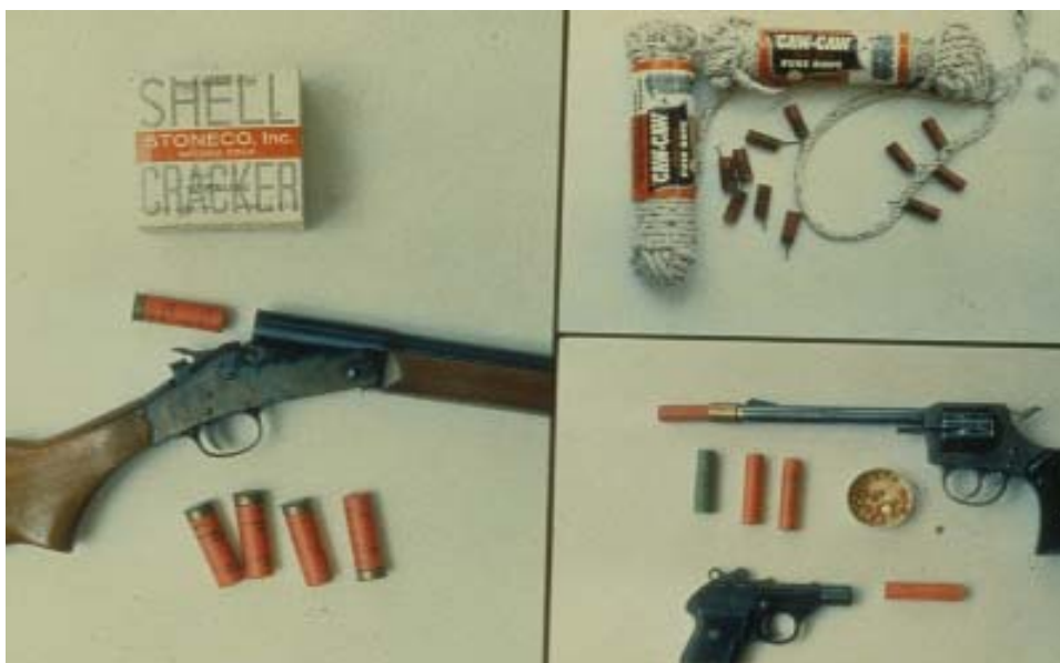
Figure 19. Pyrotechnic devices, used to haze birds. (File photo, U.S. Department of Agriculture, National Wildlife Research Center, Fort Collins, CO).
