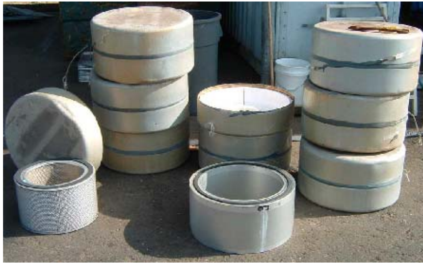
Figure 21.1 identifies the size difference between the Category One (center ground) and Category Two filters elements & filter cases prior to replacement.
