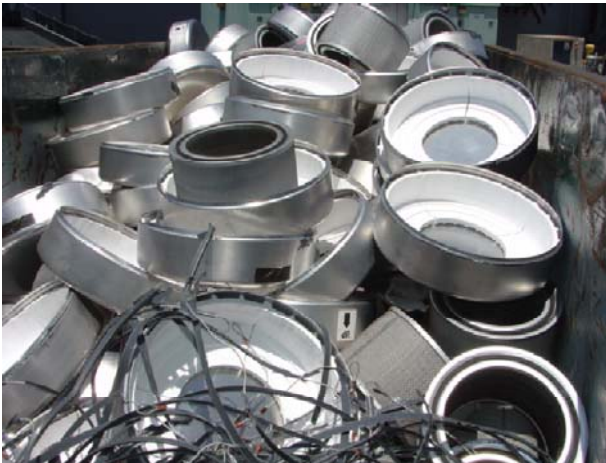
Figure 21.2 shows the segregation into a roll-off of Category Two filter elements, (filters cases and the HEPA filters).
