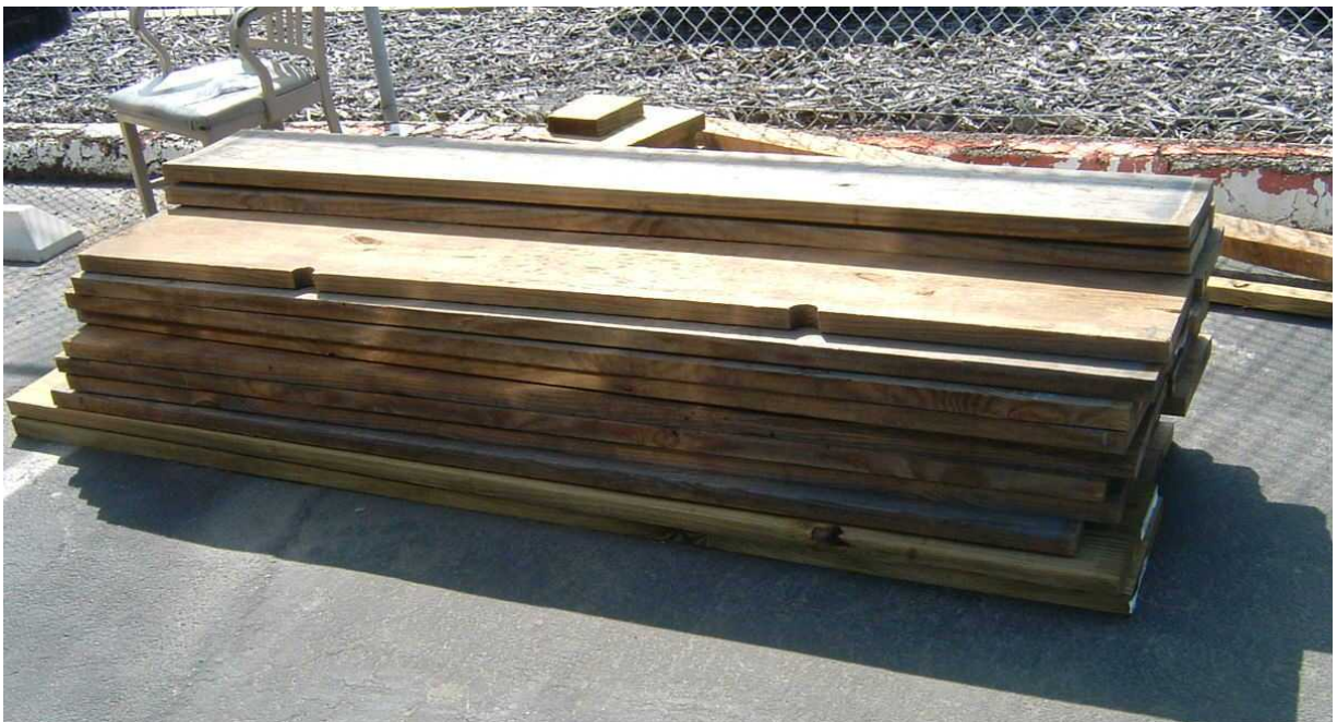
Pressure treated woods that are brown or gray. Note the color differences between the two bottom boards and the rest of the stack. Green or yellow colored pressure treated
