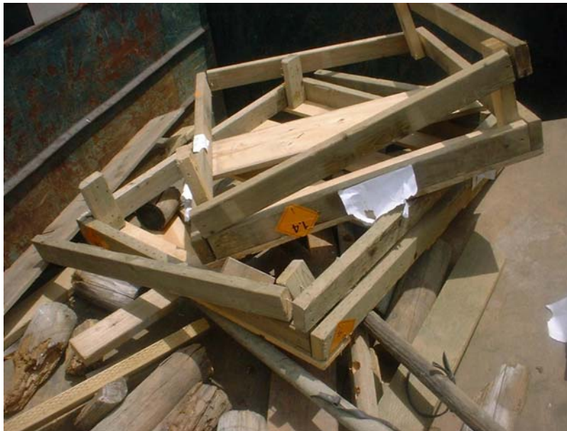
Munitions and ordnance crates and pallets. Note the green and yellow colors of the pressure treated wood commingled in with Tree Stakes.
