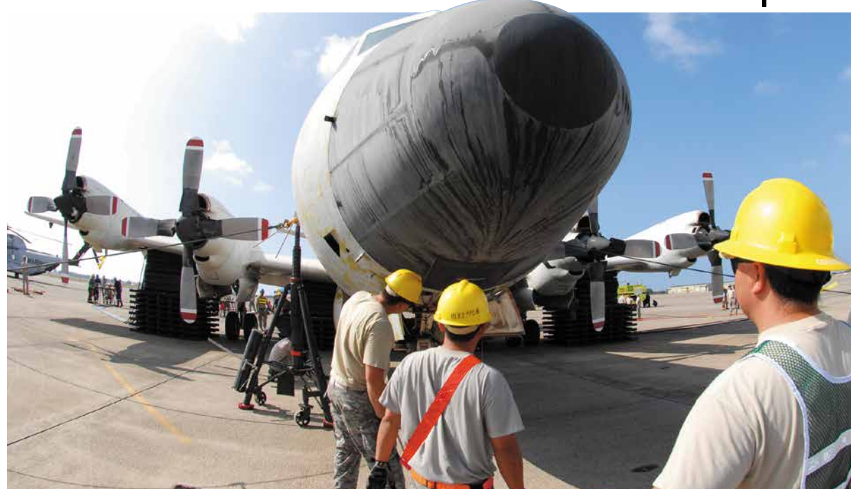
Airmen from the Hawaii Air National Guard 154th Maintenance Squadron and active duty 15th Maintenance Squadron inspect a lifted P-3 Orion aircraft during a Crash, Damaged, Disabled Aircraft Recovery training exercise, Jan. 27, at Kalealoea, Hawaii.
