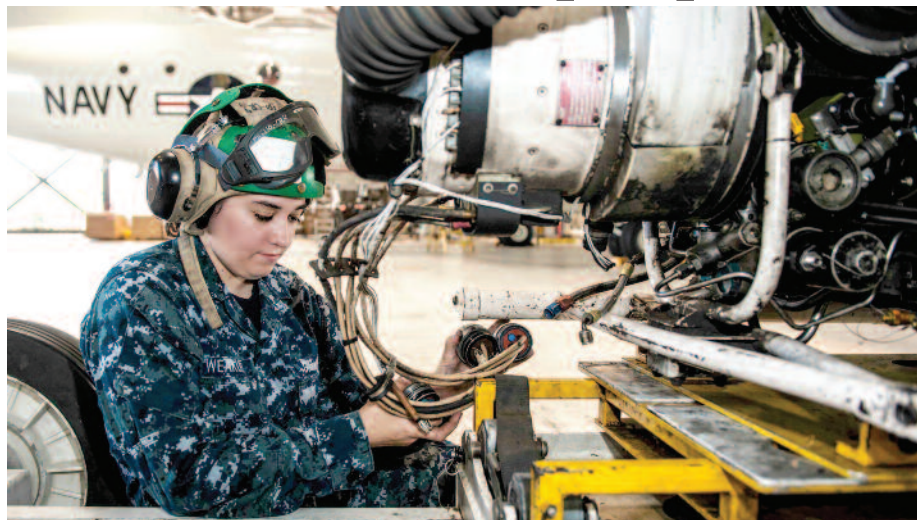
Aviation Machinist's Mate Airman Danielle Weakley, assigned to the "Golden Eagles" of Patrol Squadron (VP) 9, inspects engine three from a P-3C Orion maritime patrol aircraft as part of the squadron's advanced readiness program.
