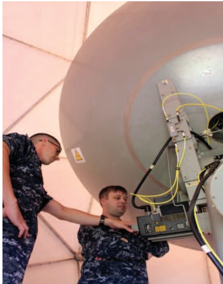
(Above) NCTAMS PAC Makalapa Tech Control personnel, Information Systems Technician 1st Class (IDW/SW) Joseph Seeley and Electronics Technician 1st Class (IDW/SW) Cameron Otejen, run initial tests on the newly installed AN/FSC-138 Navy multi-band terminal. (Above right) NCTAMS PAC Makalapa Tech Control installs the new Navy multi-band at U.S. Pacific Fleet.
