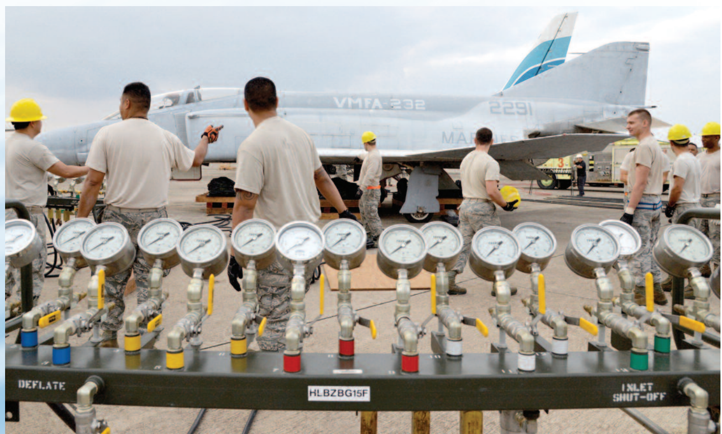
Airmen from the 15th Maintenance Squadron and Hawaii Air National Guard 154th MXS prepare airbags and control consoles in preparation to raise an F-4 Phantom II during a crash, damaged, disabled aircraft recovery exercise Jan. 14, at Kalaeloa Airport in Kapolei.
