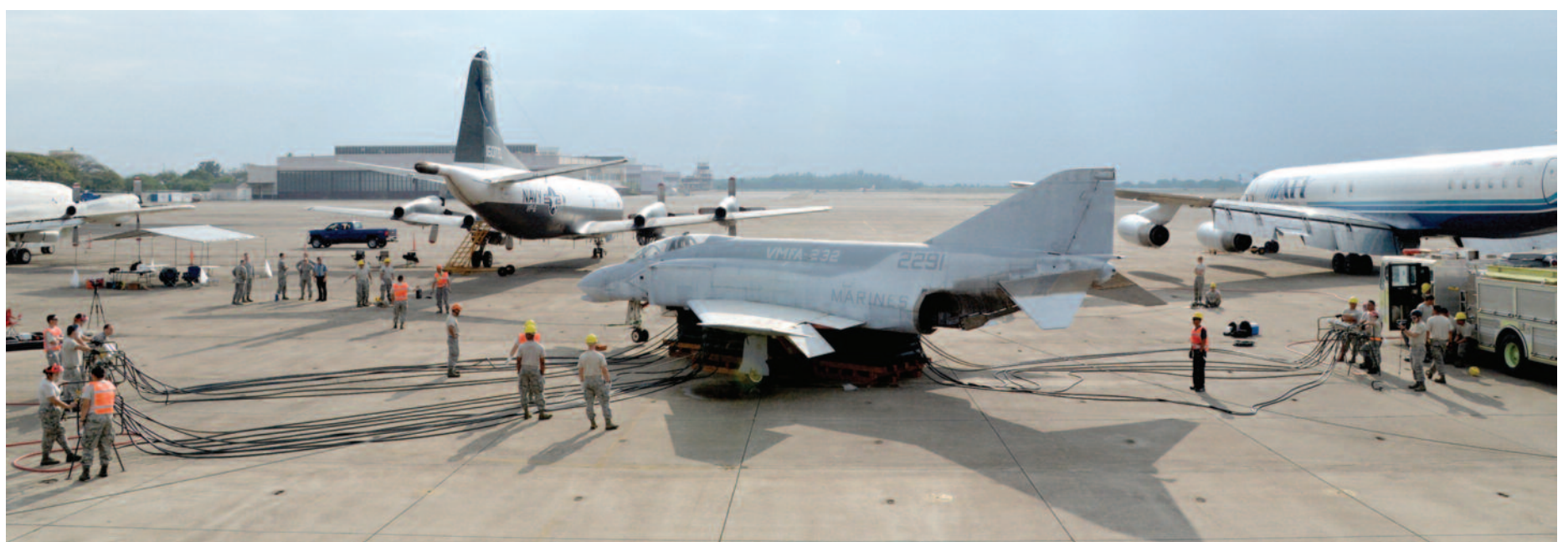
Airmen from the 15th Maintenance Squadron (MXS) and Hawaii Air National Guard 154th MXS raise an F-4 Phantom II with airbags during a crash, damaged, disabled aircraft recovery exercise Jan. 14, at Kalaeloa Airport in Kapolei. The exercise, in its third year as a joint event, was initial and refresher training for maintenance technicians, and an opportunity for a required inspection of the airbag equipment.
