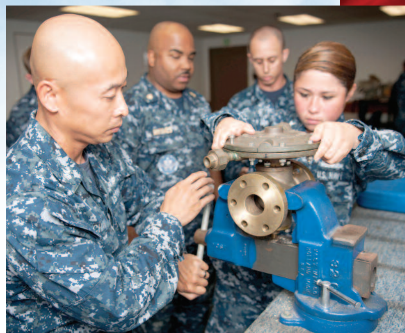
Hull Maintenance Technician 1st Class Tak Wai Chan, assigned to the guided-missile destroyer USS O'Kane (DDG 77), secures a back pressure regulating valve during the foam generation systems operations and maintenance training and labs held April 21 at the Surface Warfare Officers School, Engineering Learning Site Pearl Harbor.
