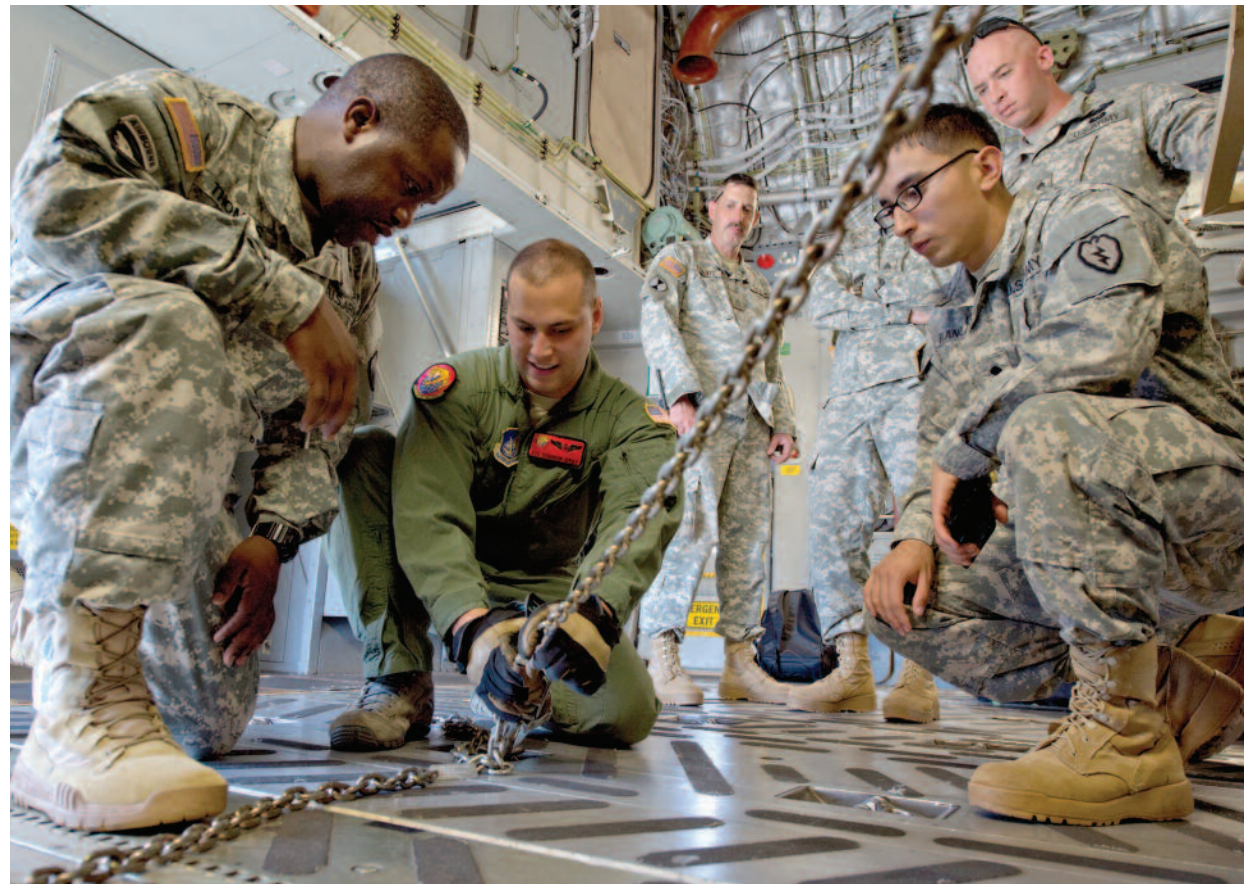
SrAirman Glenn Martin, a loadmaster from the 535th Airlift Squadron, shows Soldiers from the 2nd Brigade, 25th Infantry Division, how to use restraints to secure a tactical base of operation vehicle that is loaded in a C-17 Globemaster III on March 18 at Joint Base Pearl Harbor-Hickam. (Additional photo on page A-5.)
