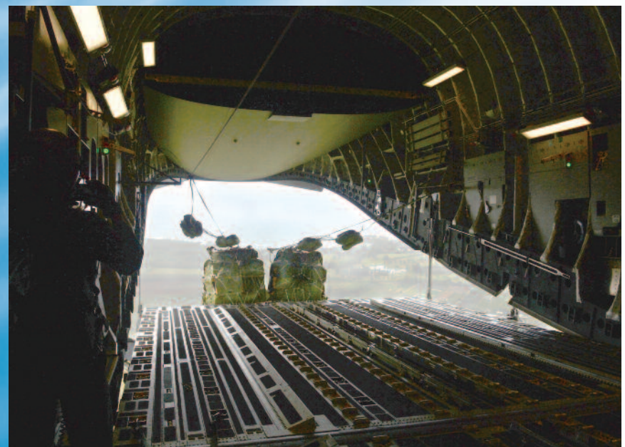
Four combat delivery systems containing 36 meals-ready-to-eat and eight ammunition containers drop out from the back of a C-17 Globemaster III from the 535th Airlift Squadron. The air drop was Feb. 27 over Kahuku Training Area.
