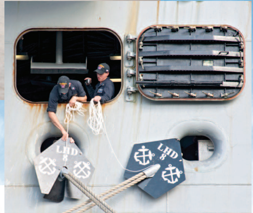
(Right) Sailors, assigned to the amphibious assault ship USS Makin Island (LHD 8), install a rat guard on a mooring line upon the ship's arrival Feb. 13 at JBPHH for a scheduled port visit.
