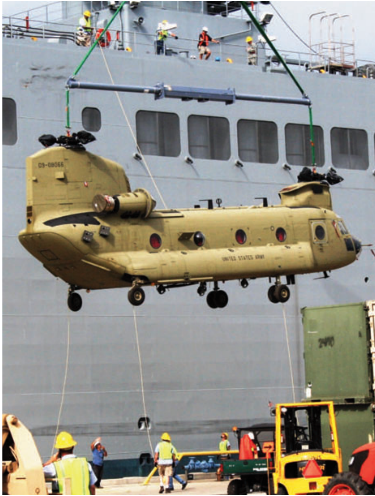
"A Chinook CH-47 helicopter is eased over the side of the USNS MENDONCA (T-AKR 303). On the pier awaiting its arrival are civilian and military personnel from FISCOPH Ocean Terminals and Navy Cargo Handling Battalion 8. Fourteen of the new multi-mission, heavy-lift helicopters were offloaded from the MENDONCA on 18 November. Mechanics reattached their propellers and prepared them for flight, and they were flown to their new home at Wheeler Army Airfield."
