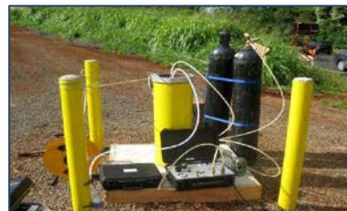
Groundwater monitoring well being sampled
