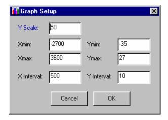
This window is used to set the scale and grid for the graphical display. The Y Scale field is used to stretch or shrink the vertical Y axis. The <u>Xmax</u> and <u>Xmin</u> fields set the maximum and minimum stations of the grid. The Ymax and <u>Ymin</u> fields set the
