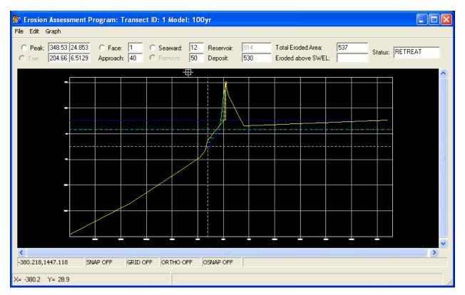
The erosion assessment analysis is performed graphically by selecting points along the profile. The program requires the user to select these points. The following step-by-step instructions outline the procedures for performing a frontal dune erosion treatment within CHAMP. Instructions consider frontal dune erosion treatment for ground profiles where the dune crest is: A) above; and B) below the 1% or 0.2% annual chance SWEL.
