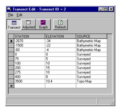
Transect station and elevation data can also be imported by selecting the <u>Import</u> menu item under the <u>File</u> menu. CHAMP only allows importing comma-delimited text files (.csv) for importing station and elevation data for a transect. This works much the same as importing project data described above.
