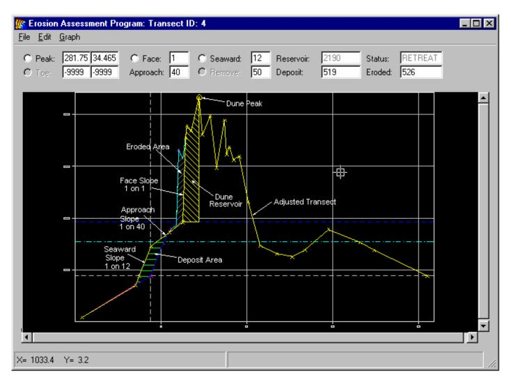
Check the <u>Deposit</u> field to see if it matches the <u>Total Eroded Area</u> field. If they match or are close, the erosion treatment is complete. If they are not close, the selection of the seaward slope can be repeated until the deposition area matches the eroded area.
