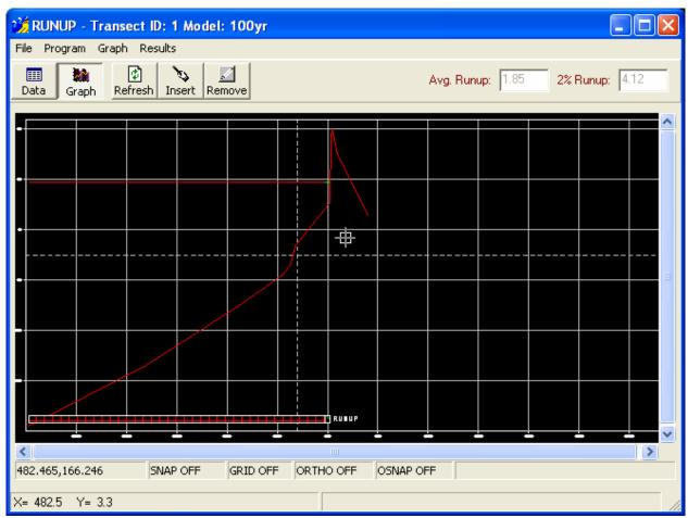
This plot shows the profile used in the runup analysis in red and the computed runup elevation (average computed runup depth plus SWEL) as a red dashed line. Click on the Data button to return to the RUNUP input window
