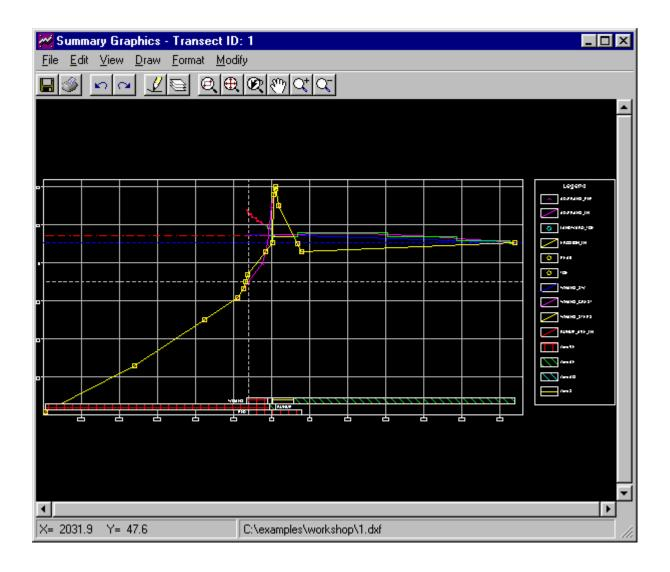
This plot displays all of the results from each program within CHAMP. Each feature can be turned off or on by selecting the <u>Layers</u> item under the <u>Format</u> menu. The graphic can be printed by clicking on the <u>Print</u> menu item under the <u>File</u> menu.
