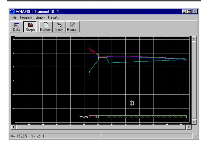
A hatched color-coded bar at the bottom of the plot represents the different zones:
