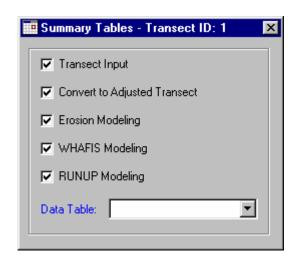
Each phase or program of CHAMP is listed. When a program has been completed, a check mark will be shown next to that program. Should your modeling effort be interrupted for some reason, this feature can be used to keep track of all completed analyses and track the remaining analyses to be completed for each transect.
