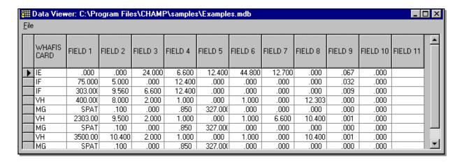
**Part 2** shows the controlling wave heights, spectral peak wave period, and wave crest elevations for the data entry points and all WHAFIS interpolated values.
