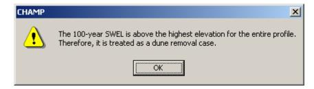
Click on OK to remove the dune and follow the instructions above for selecting the toe and drawing the eroded profile.
