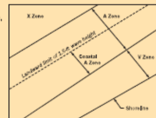
Plan view showing a Coastal A zone landward of a V zone (source: ASCE 24-05).
