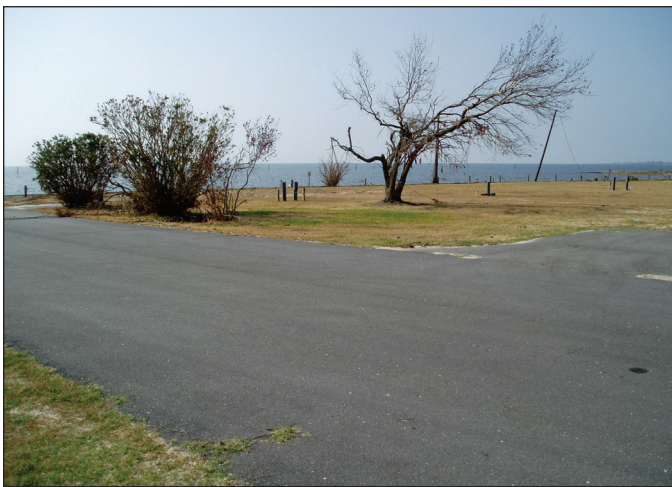
Figure 10. The site on the left is mapped Zone AE, and lies directly along the Gulf of Mexico shoreline. Limited obstructions to waves indicate the site could be classified as a Coastal A zone. The site on the right is over ½ mile from the Gulf shoreline, is mapped as Zone AE, and has a base flood stillwater level sufficient to support >1.5' wave heights – but obstructions to waves (e.g., trees and other buildings between the site and the shoreline) and distance from the source of flooding would indicate the area is not a Coastal A zone.
