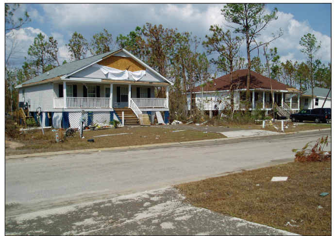
Figure 10. The site on the left is mapped Zone AE, and lies directly along the Gulf of Mexico shoreline. Limited obstructions to waves indicate the site could be classified as a Coastal A zone. The site on the right is over ½ mile from the Gulf shoreline, is mapped as Zone AE, and has a base flood stillwater level sufficient to support >1.5' wave heights – but obstructions to waves (e.g., trees and other buildings between the site and the shoreline) and distance from the source of flooding would indicate the area is not a Coastal A zone.
