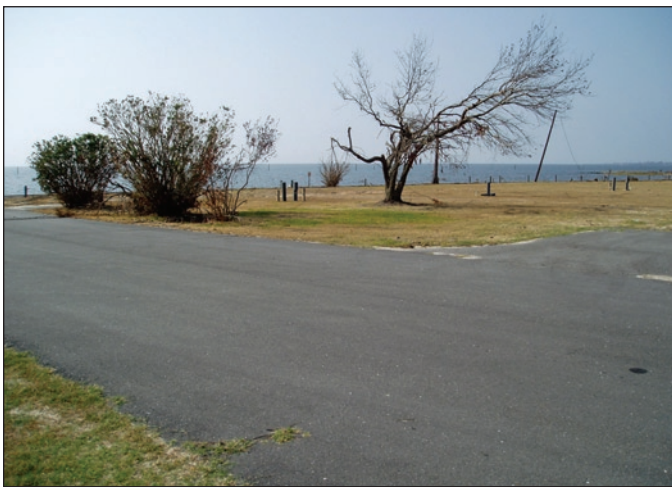
Figure 10. The site on the left is mapped Zone AE, and lies directly along the Gulf of Mexico shoreline. Limited obstructions to waves indicate the site could be classified as a Coastal A zone. The site on the right is over 1/2 mile from the Gulf shoreline, is mapped as Zone AE, and has a base flood stillwater level sufficient to support >1.5' wave heights – but obstructions to waves (e.g., trees and other buildings between the site and the shoreline) and distance from the source of flooding would indicate the area is not a Coastal A zone.
