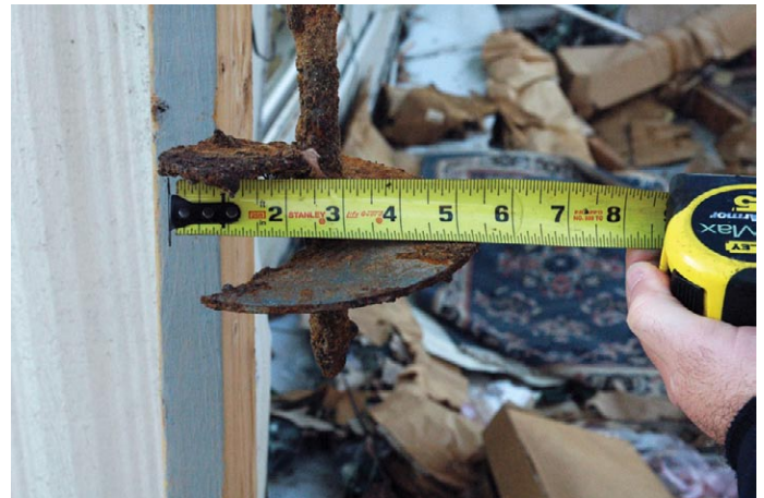
This 4-foot-long ground anchor with a 6-inch diameter helix pulled out of the soil. Soils in the area consisted of loose sands. Longer anchors with larger diameter helices would have been a better choice for this soil type. The anchor spacing at this home was approximately 10 feet.
