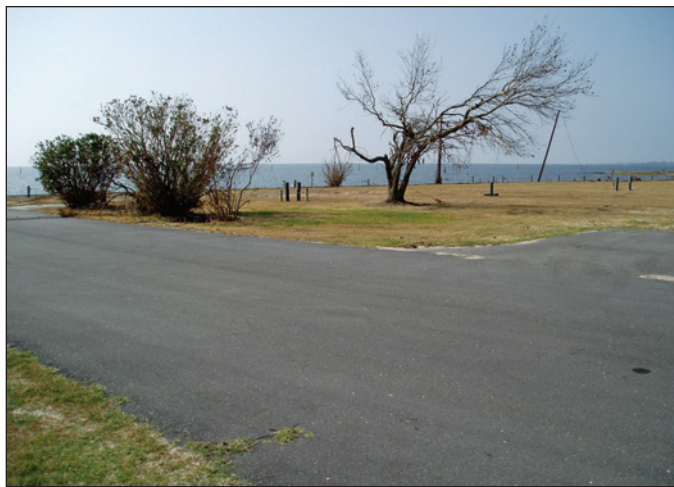
Figure 10. Although the site on the left is mapped Zone AE, proximity to the Gulf of Mexico shoreline and limited obstructions to waves indicate the site could be classified as a Coastal A Zone. The site on the right is over 4,000 feet from the Gulf shoreline and over 1,000 feet from the bayou, mapped as Zone AE, and has a base flood stillwater level sufficient to support >1.5-foot wave heights – but obstructions to waves (e.g., trees and other buildings between the site and the shoreline), and distance from the sources of flooding would indicate the area is not a Coastal A Zone.
