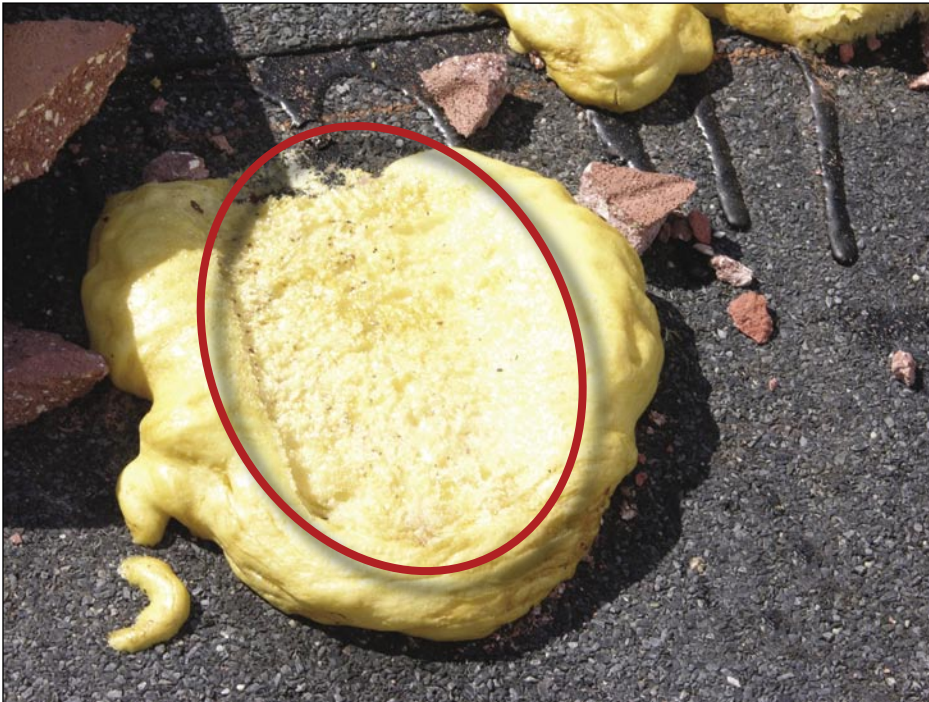
Figure 5-44. In this photo, the portion of the paddy that made contact with the tile is clearly visible (Punta Gorda Isles).
