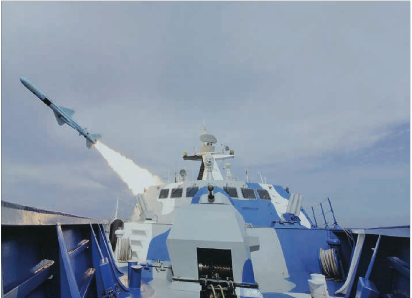
Houbei-class 002 Fast Attack Missile Craft test fires C-803 antiship missile (Global Military Review)
