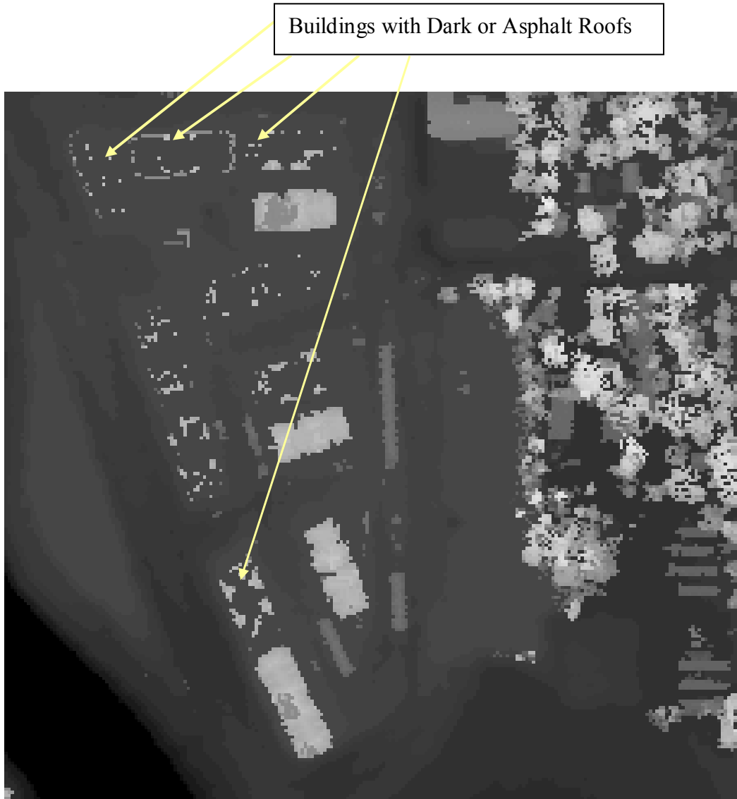
Figure 42 — No LIDAR data collected for certain buildings with dark roofs (i.e., tar or asphalt). Tile q29095g44.
