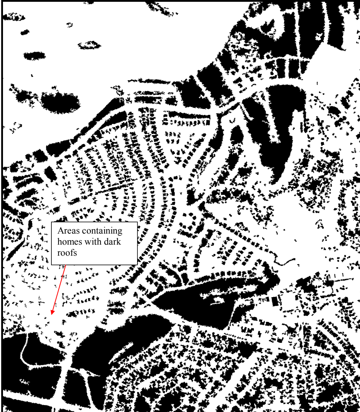
Figure 41 — Footprints of structures extracted in tile q30095a24. As result, there is poor penetration of laser beams in foliage, most buildings in forested area are merged. Forested areas look like huge clusters versus individual stands of tree.
