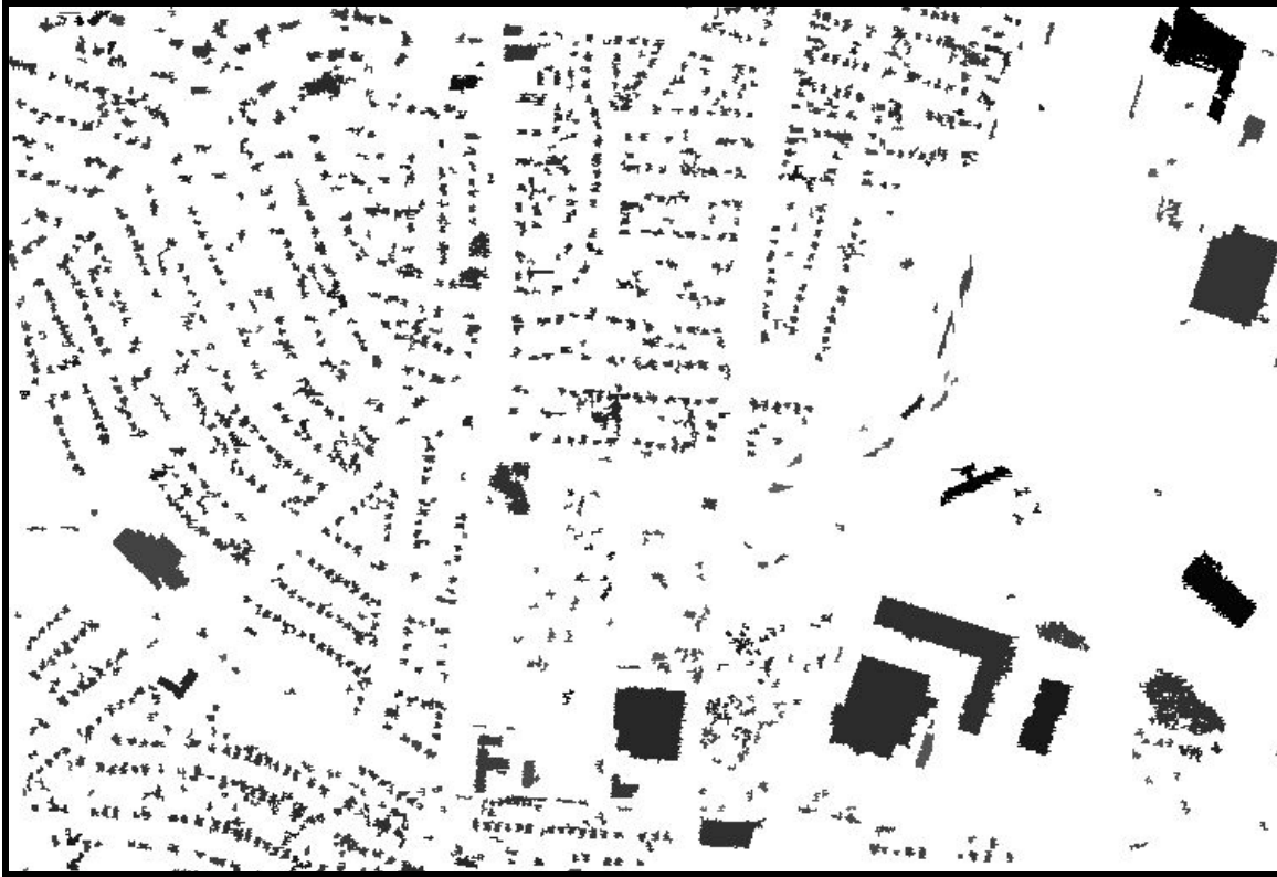
Figure 35 — Footprints of 1,220 Objects and Structures Automatically Extracted for Tile 208NE04 of Highly Populated Prince George's County, MD.
