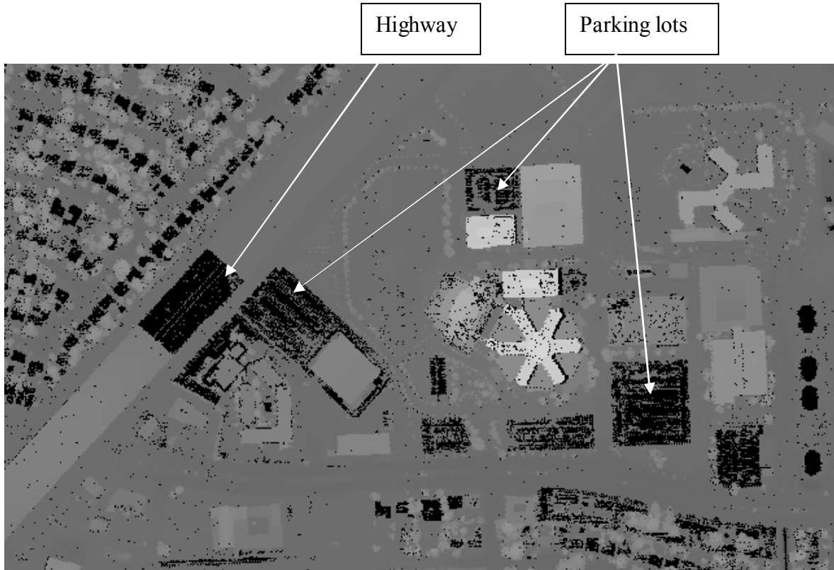
Figure 43 — Z_minimal for part of tile q29095f52 (center of bottom part), Harris County, TX before filling holes. All dark areas are areas without LIDAR data. These dark areas include the part of highway, parking lots and homes in this tile.
