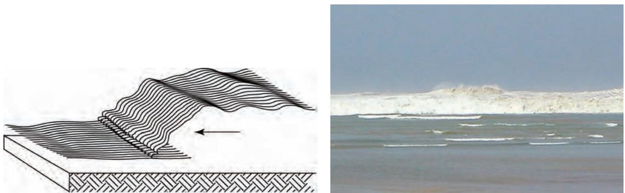
Figure 2-5 Sketch of a bore and photo of the 1983 Nihonkai-Chubu Tsunami showing the formation of a bore offshore (Photo from Knill, 2004).
