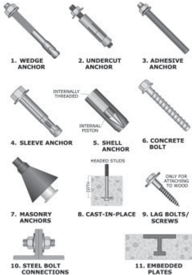
Figure 127: Types of anchors.
