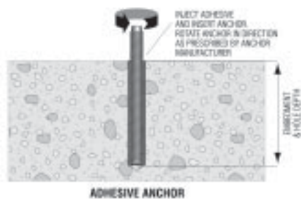
Figure 131: Adhesive anchor installation.
