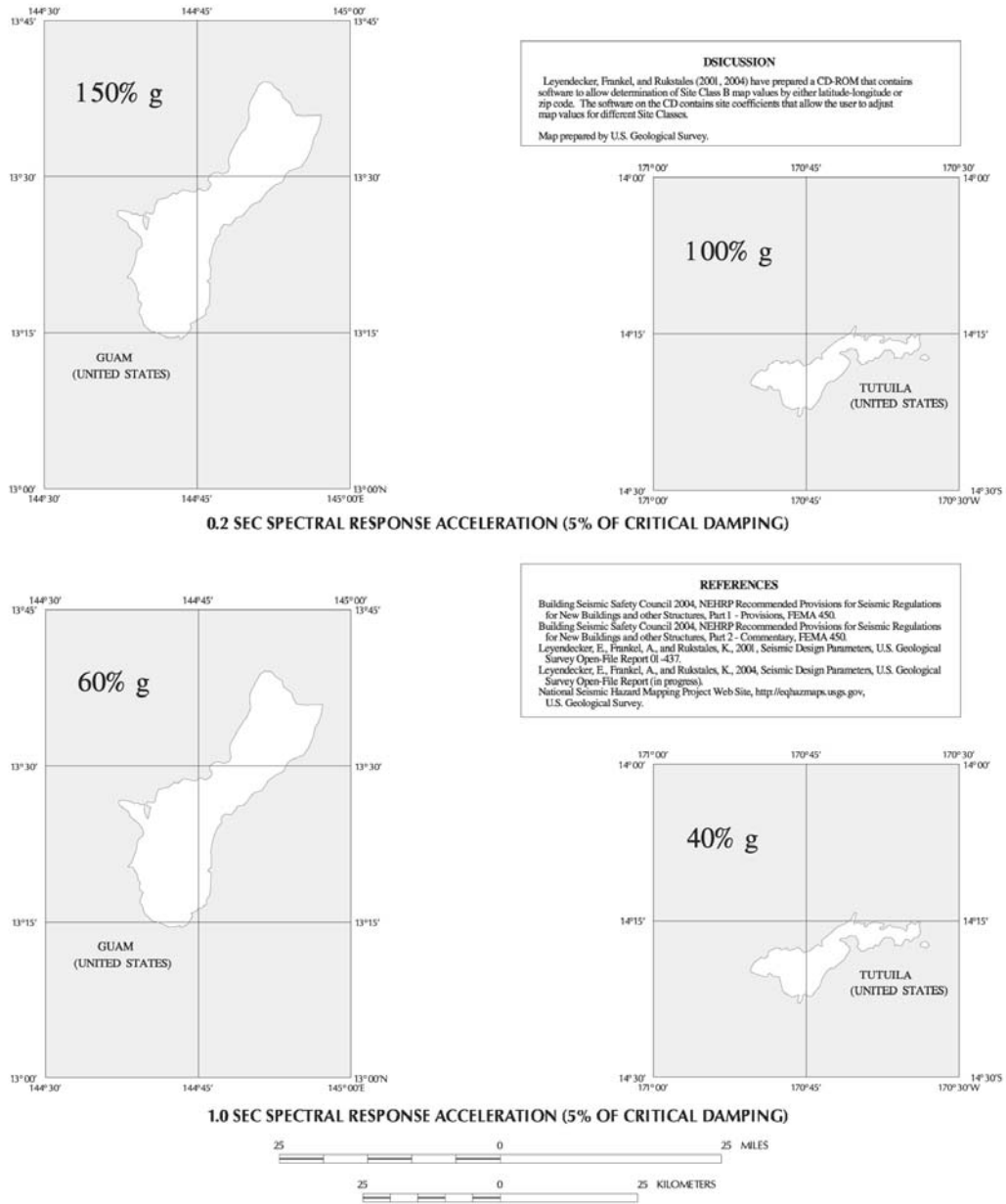
FIGURE 3.3-14 MAXIMUM CONSIDERED EARTHQUAKE GROUND MOTION FOR GUAM AND TUTUILA OF 0.2 AND 1.0 SEC SPECTRAL RESPONSE ACCELERATION (5% OF CRITICAL DAMPING), SITE CLASS B
