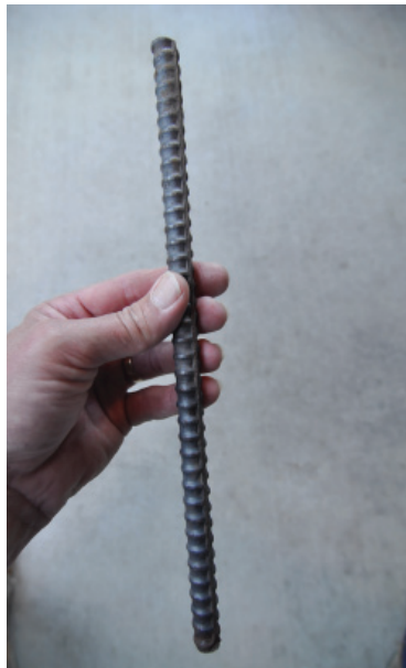
■ Figure 26. A piece of #4 bar (a steel reinforcing bar that is 4/8 inch in diameter).
