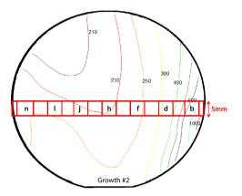
Fig. 3. Resistivity map in units of  $\Omega/\Box$  for growth #2. The gradient across the 76-mm wafer is a result of varying strain in the InGaAs channel and InAlAs barrier layers. The wafer was cleaved into  $5 \times 5 \text{ mm}^2$  squares, as indicated.
