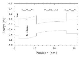
Fig. 8. Calculated band structure of  $In_{0.8}Ga_{0.2}As/In_{0.7}Al_{0.3}As$  QW. The conduction band offset is 316 meV; the electron sheet density is  $1.4 \times 10^{12}/cm^2$ .
