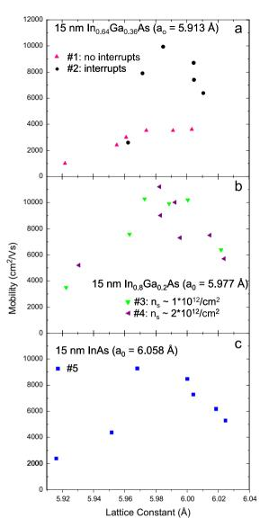
**Fig. 6.** Room-temperature mobility as a function of buffer layer lattice parameter for samples from all five growths. Peak mobilities are achieved for lattice parameters of 5.97–6.00 Å. Mobility decreases for smaller lattice parameters due to roughness in the buffer layers. For larger lattice parameters, mobility decreases due to high tensile strains (> 2%) in the InAIAs barriers.
