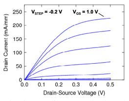
**Fig. 7.** FET drain characteristics for  $In_{0.64}Ga_{0.36}As$ -channel HEMT in tension (growth #2) with  $L_G$ =100 nm and  $W_G$ =31 µm.
