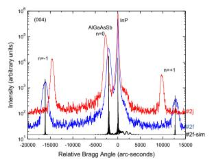
**Fig. 4.** X-ray diffraction data for samples #2f and 2j and simulation for 2f. The lattice parameter of the buffer layer (and the strain in the channel and barrier layers) is extracted from the peak separations.
