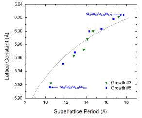
**Fig. 5.** Buffer layer lattice parameter vs. superlattice period for growths #3 and 5. Solid line is calculated (see text).
