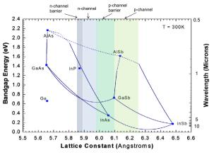
Fig. 1. Energy gap vs. lattice parameter showing regions usually used for channels and barriers in n- and p-channel FETs.
