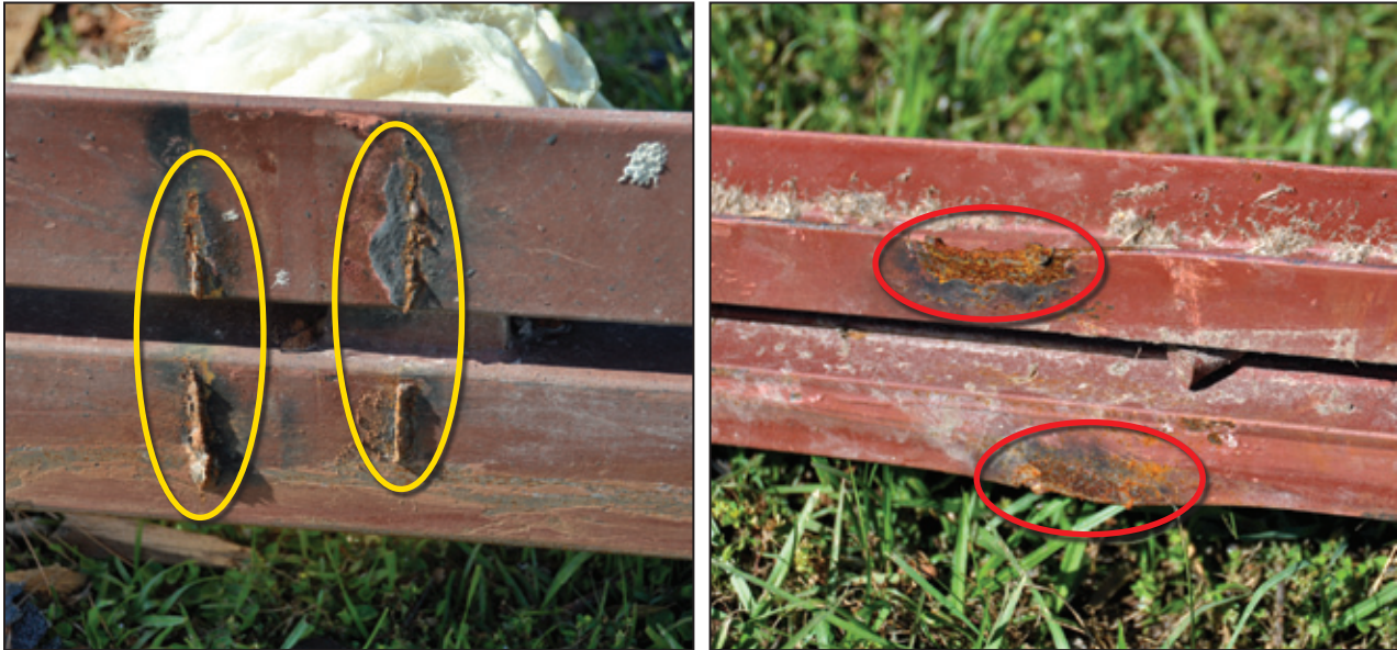
Figure 6-20: The yellow ovals on the left photograph show weld remnants where a joist was attached to the girder. The red ovals on the right photograph show weld remnants where a joist was attached to a bearing plate at a bond beam (Tuscaloosa, AL).
