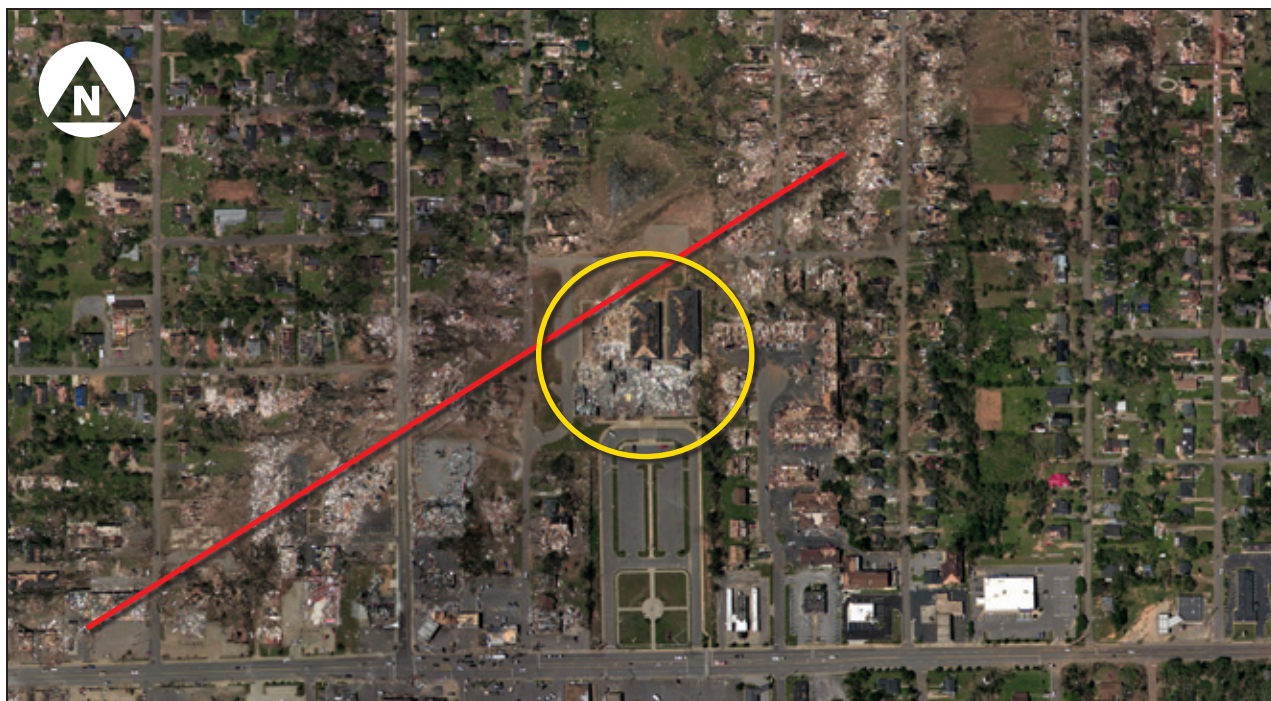
Figure 6-3: Aerial view of tornado track in vicinity of Alberta Elementary School (yellow circle). The center of the damage swath is approximated by the red line 1 (Tuscaloosa, AL).
