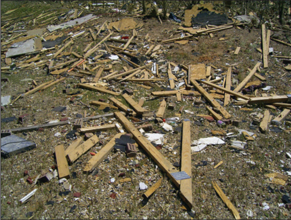
Figure 3-6: Example of small- and medium-sized missiles commonly observed by the MAT (photograph taken near an apartment complex in Tuscaloosa, AL)
