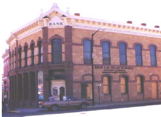
Example of a Bearing Wall Structure
