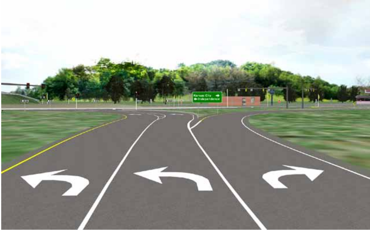
Figure 176. Illustration. Advanced pavement markings and guide signs from the off-ramp. (83)
