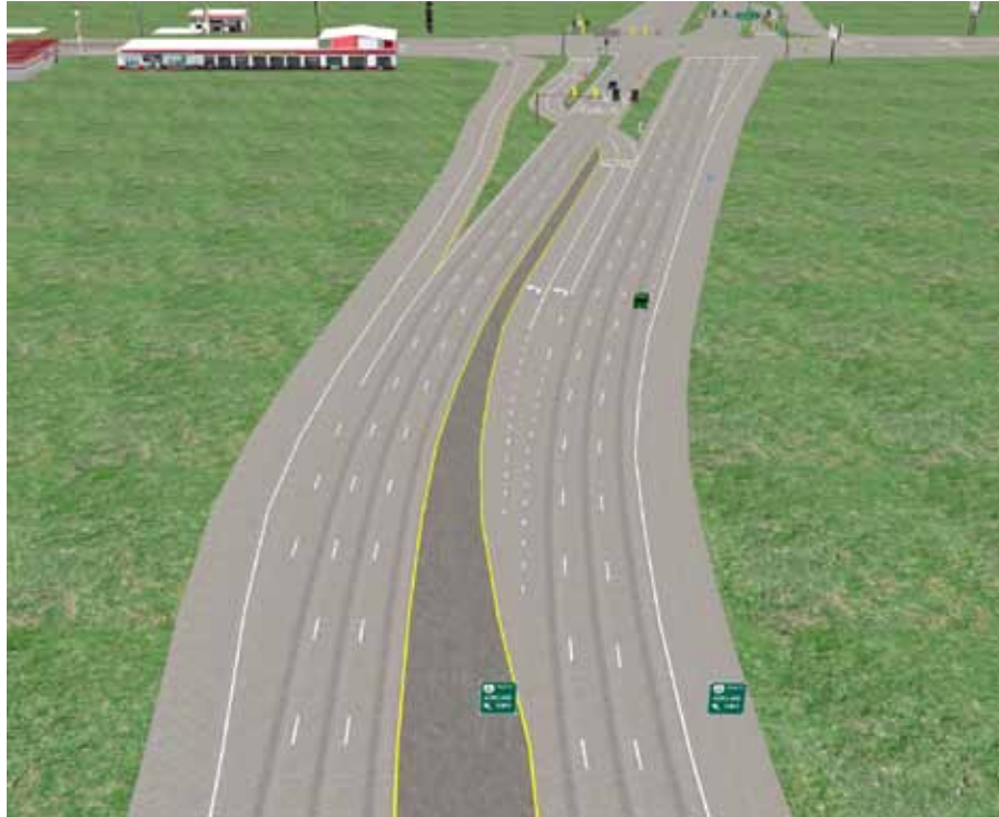
Figure 188. Illustration. Left-turn crossover movement view, as shown in a DLT intersection driver simulator.
