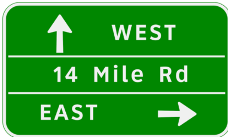
Figure 69. Illustration. Alternate major street advanced guide sign.
