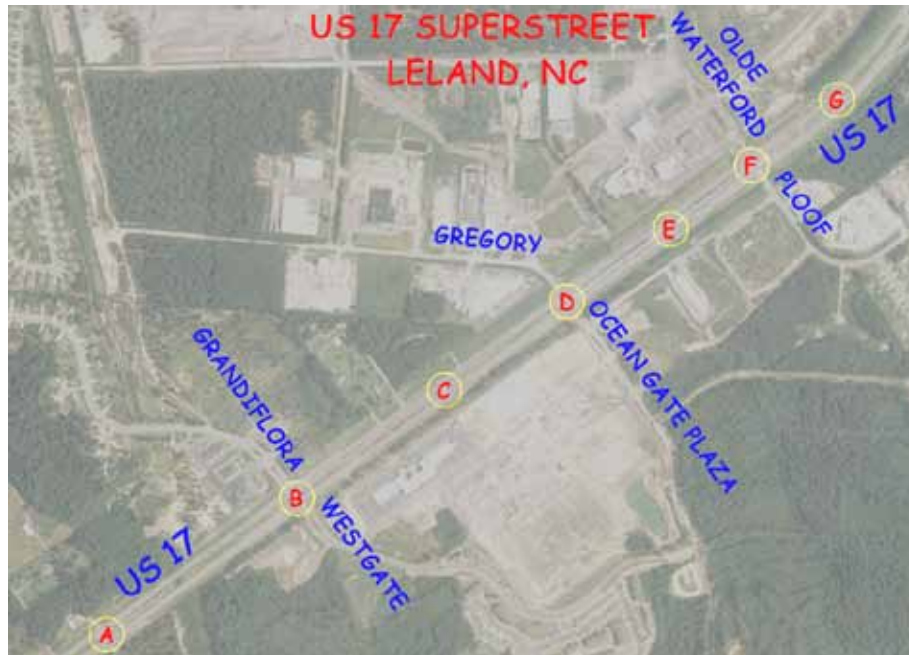
Figure 121. Photo. RCUT treatment at three intersections on U.S. Route 17 in Leland, NC.
