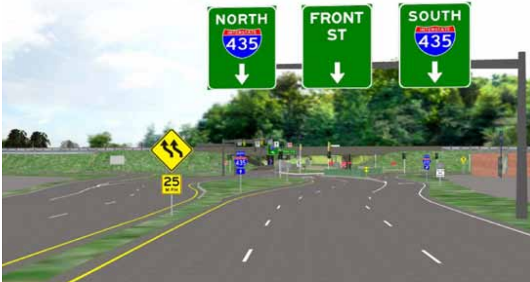
Figure 174. Illustration. Overhead signing proposed for the planned DCD interchange ahead of the crossover in Kansas City, MO. (83)
