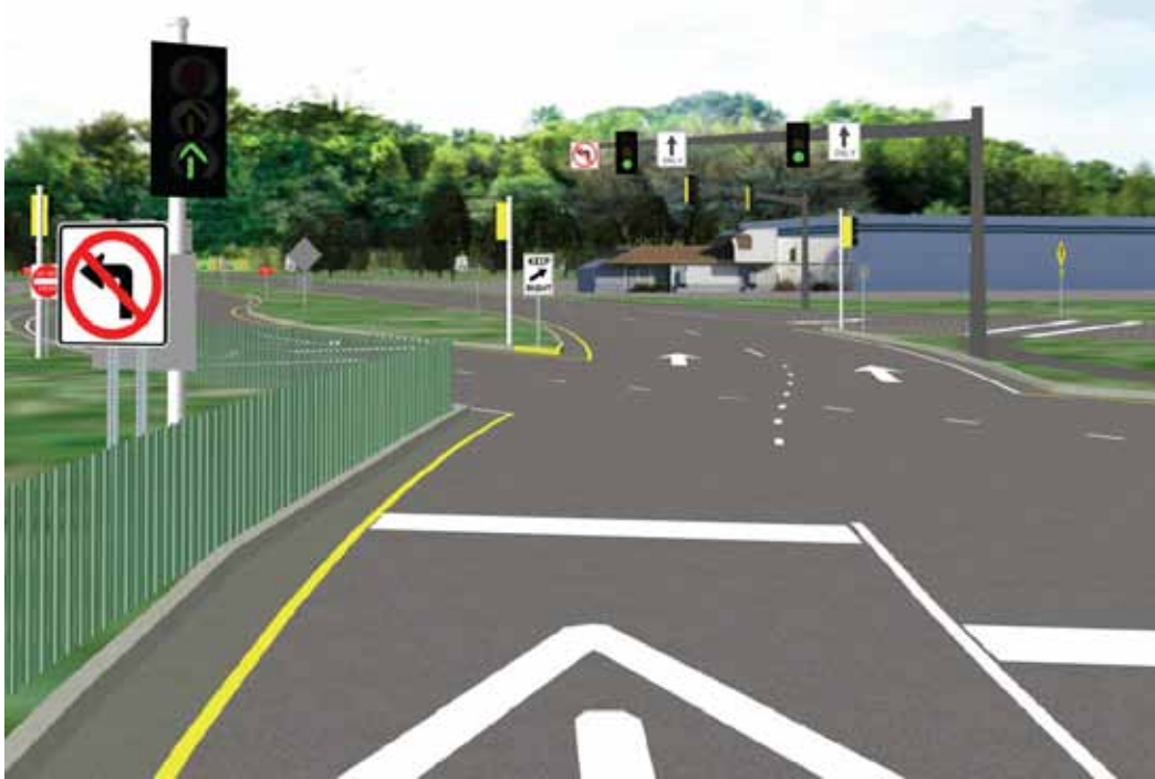
Figure 170. Illustration. Green arrows, overhead lane usage, and skip markings proposed for the planned DCD interchange in Kansas City, MO. (83)
