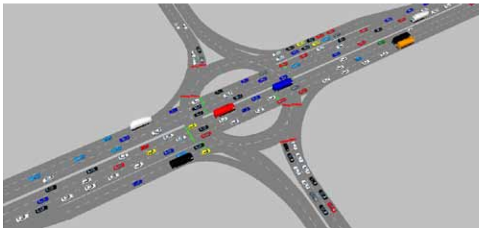
Figure 145. Photo. Typical hamburger intersection movements. (75)
