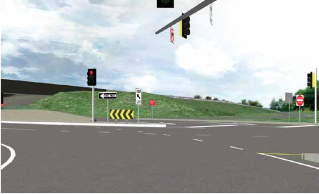
Figure 171. Illustration. “Wrong Way” and “One Way” signs proposed for the DCD interchange in Kansas City, MO. (83)
