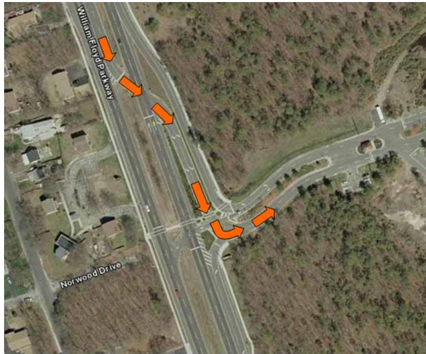
Figure 3. Photo. Left-turn crossover movement at a three-legged partial DLT intersection in Shirley, NY.
