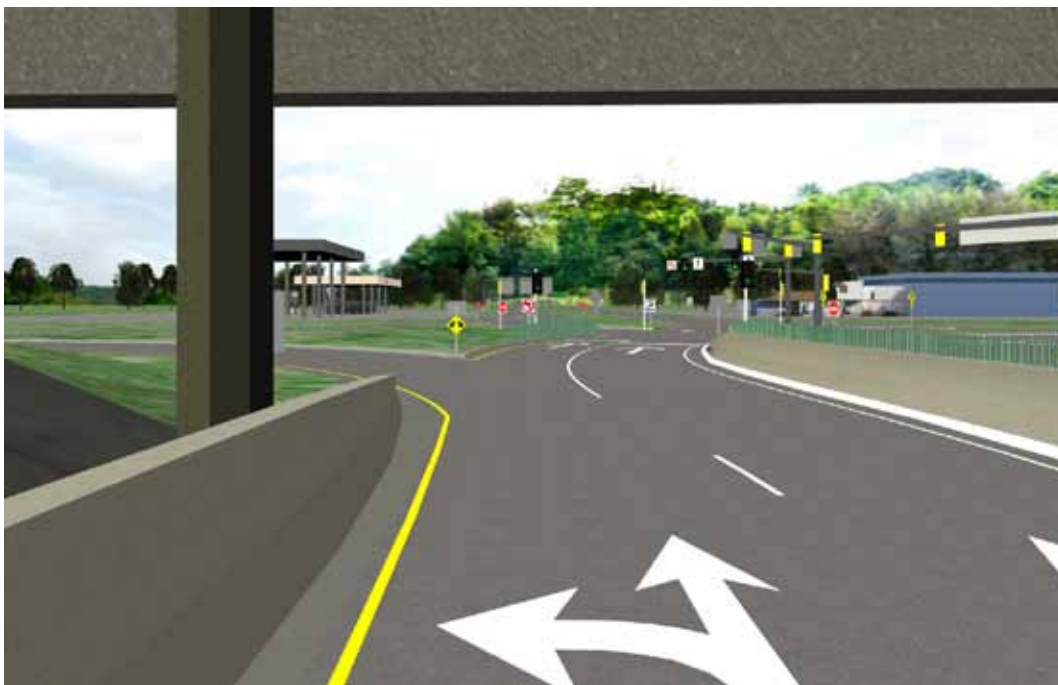
Figure 175. Illustration. Signing and pavement marking proposed for the planned DCD interchange ahead of the left turn off-ramp in Kansas City, MO. (83)
