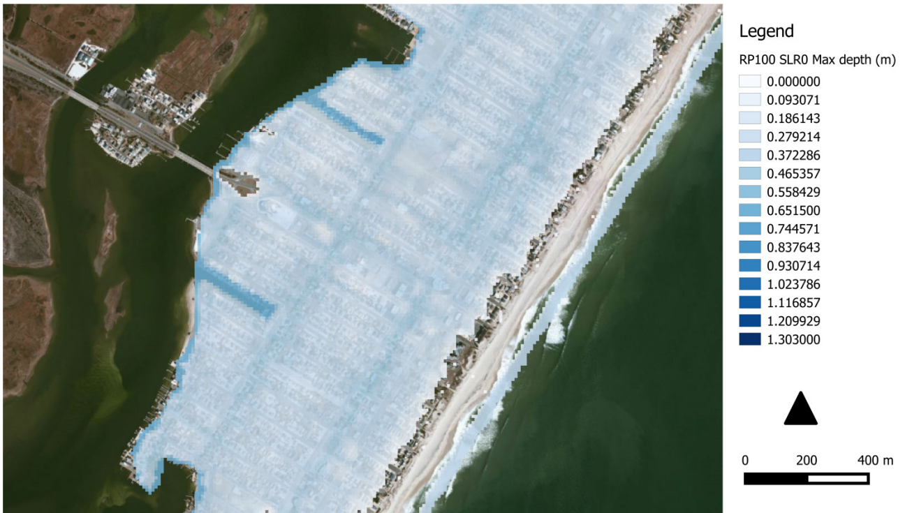
Figure 6.16: Map of the maximum flood depth for the scenario RP 100 y, SLR 0 ft
