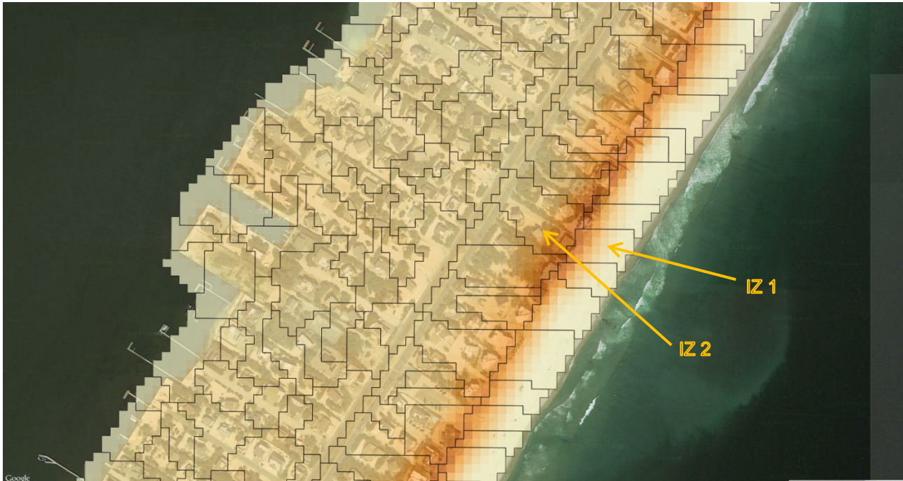
Figure 6.14: View of the computational elements (IZs, black polygon lines) generated by AccData
