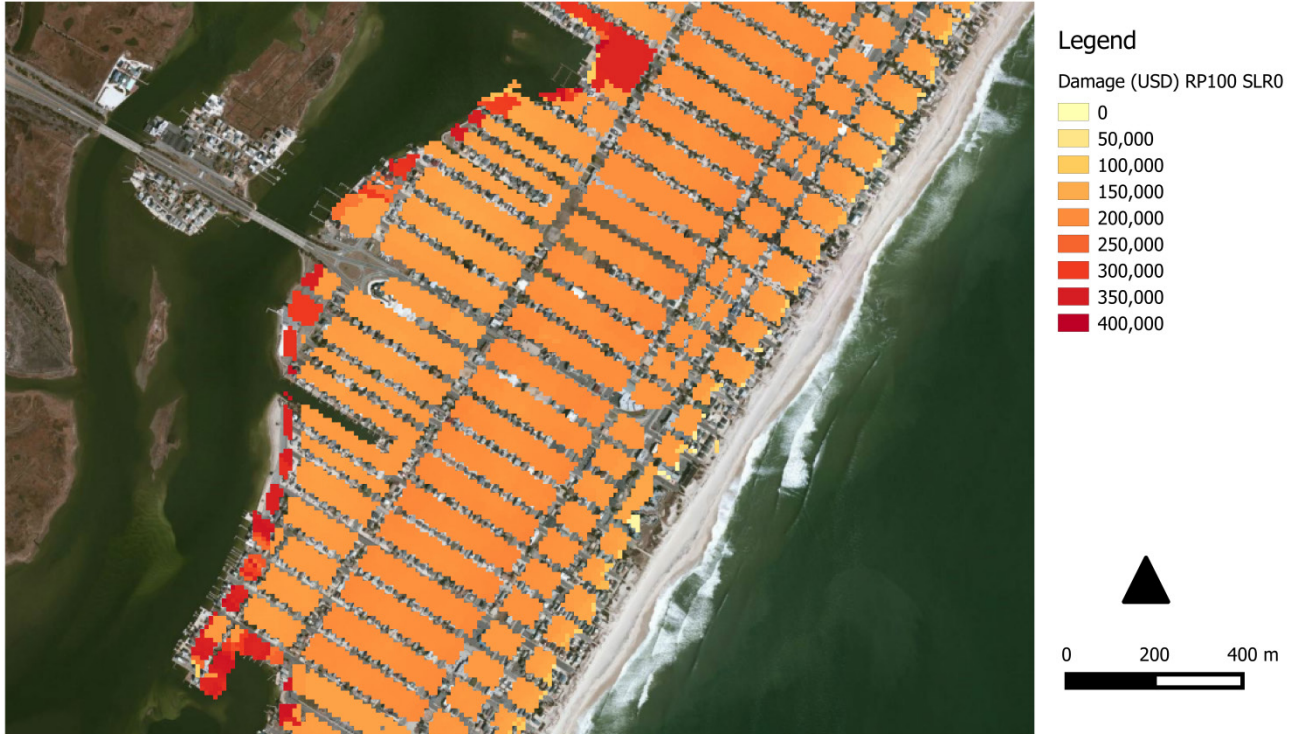
Figure 6.28: View of the calculated damage for RP 100 (SLR 0 ft). Note that the damage value is each grid cell is the damage in the corresponding parcel, not the damage per cell
