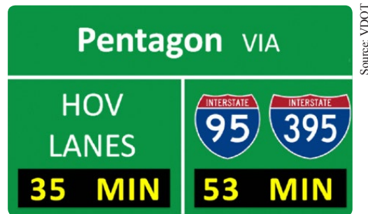
Figure 11. Illustration. A dynamic traveler information sign indicates the amount of time it will take to reach a destination via high-occupancy vehicle lanes versus normal travel lanes.
