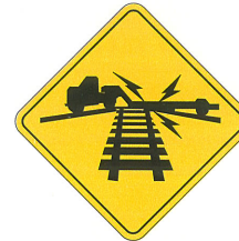
LOW GROUND CLEARANCE ON TRACK (W10-5)
