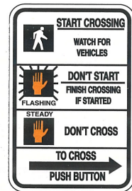
PEDESTRIAN PUSH BUTTON/PEDESTRIAN SIGNAL MEANINGS (R10-3b)
