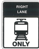
LIGHT RAIL ONLY LANE (R15-4a)
