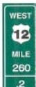
ROADWAY IDENTIFICATION AND MILE MARKER MEASURED TO ONE-TENTH OF A MILE* (D10-8)
