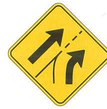
ENTERING ROADWAY ADDED LANE (RIGHT)* (W4-3a)
