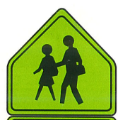
SCHOOL CROSSWALK (S1-1 and W16-7p)
