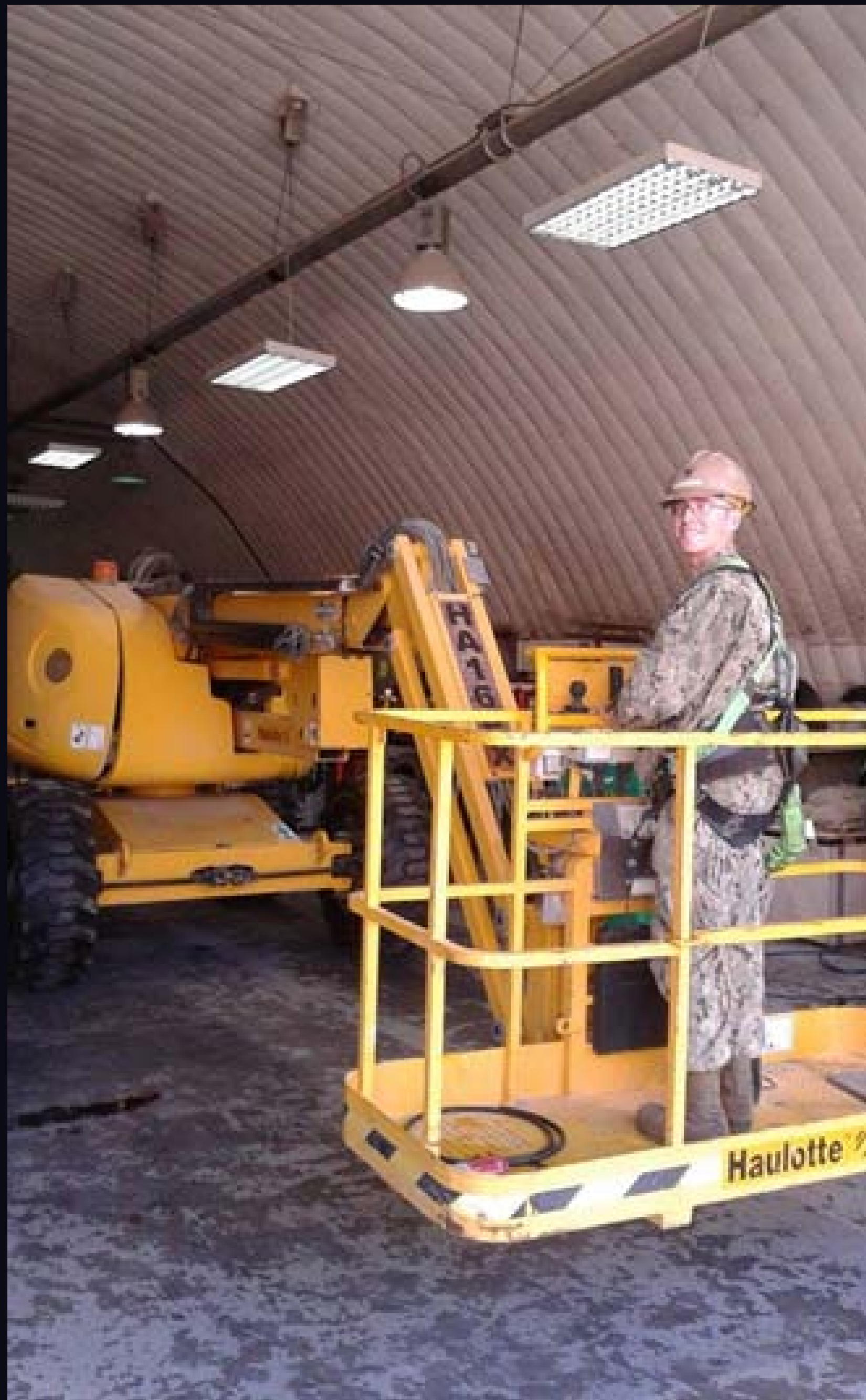
At the Transportation Maintenance Shop, Equipment Operator Third Class Benjamin Primozic conducts an operational check on the Haulotte man-lift after a tire change to ensure proper mobility and safe operation of the equipment. (U.S. Navy photo by CE1 Travis Harvey)
