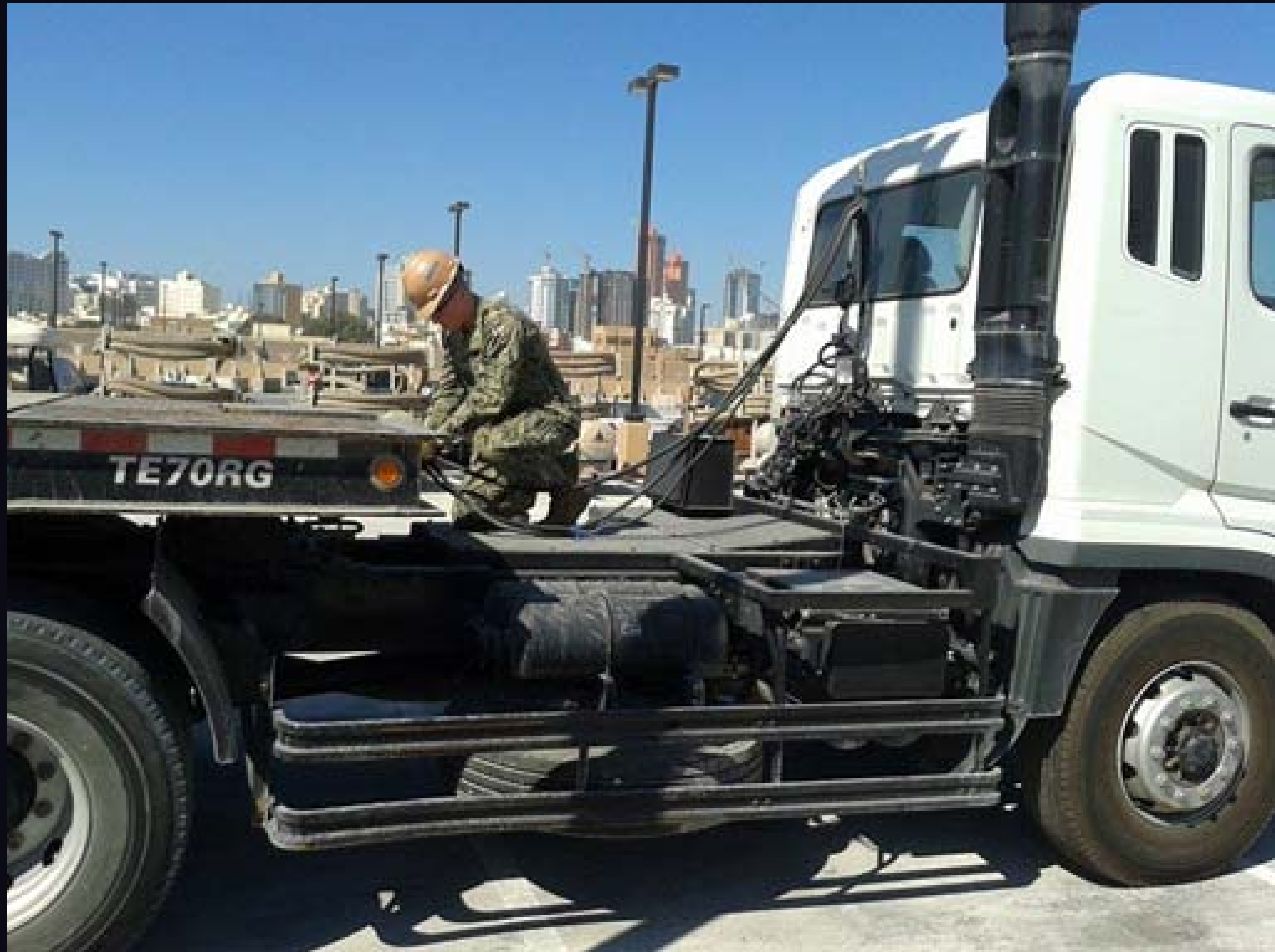
As part of a pre-start inspection procedure EOCN Justin Peters checks an air connection on a tractor trailer. After its successful completion, he was able to move the equipment from NSA 1 to NSA 2. (U.S. Navy photo by CE1 Travis Harvey)
