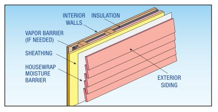
Figure 9-9. Example of wood siding on a wood-framed house.
