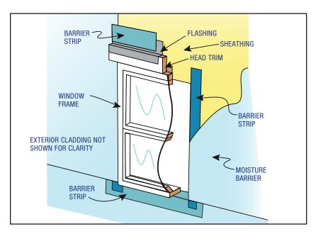
Figure 9-5. Window flashing details.
