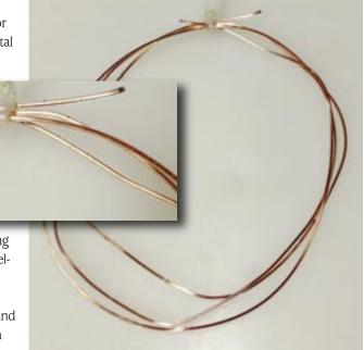
Copper torpedo guidance wire with plastic coating intact after 45 days. INSET: After 45 days, only the tips of the copper wire experienced any corrosion.
