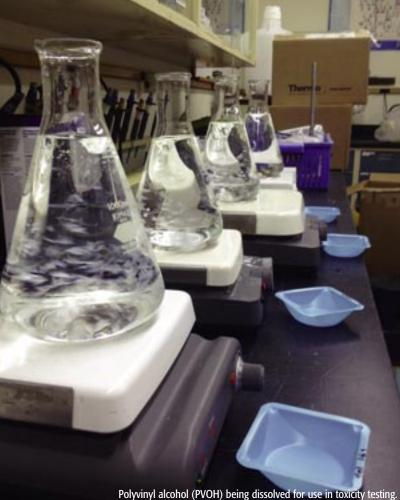
Polyvinyl alcohol (PVOH) being dissolved for use in toxicity testing. Brandon Swope
